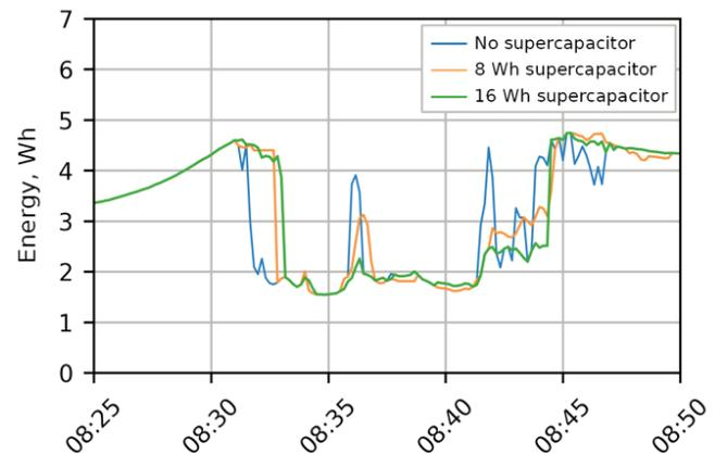
Fig. 12. Time interval 08:25–08:50 of the analyzed production curve, presenting basic generation flow and influence of 8 Wh and 16 Wh supercapacitor energy banks on the DC output.
