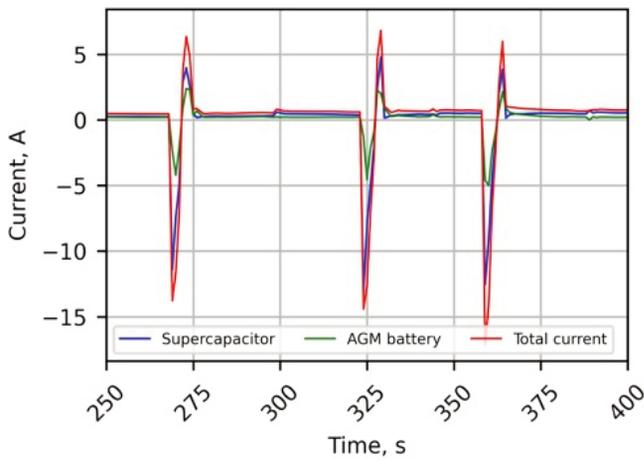
Fig. 16. Values of the current flowing in a hybrid storage system with a capacity of 65 Ah connected to a standard 2 kW PV installation.
