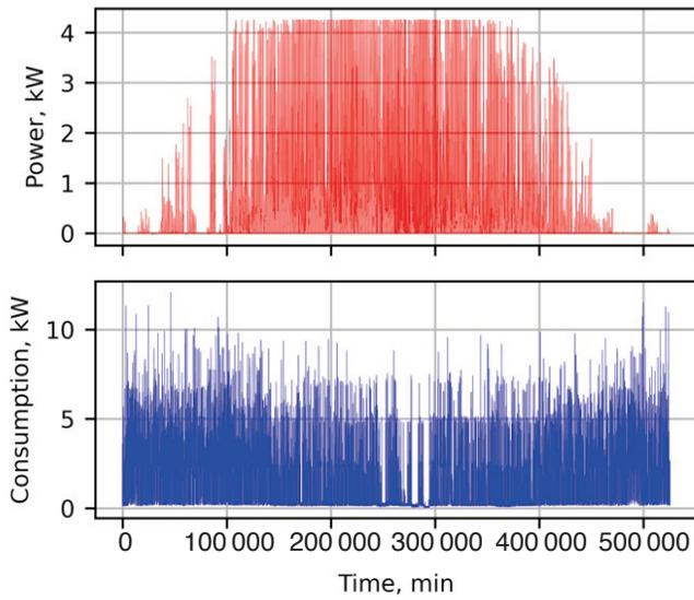
Fig. 5. Average hourly PV generation and power consumption by the residential building.
