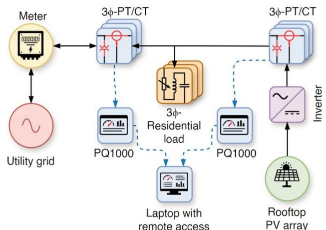
Fig. 3. Simplified diagram of the designed residential generation and consumption logging system.
