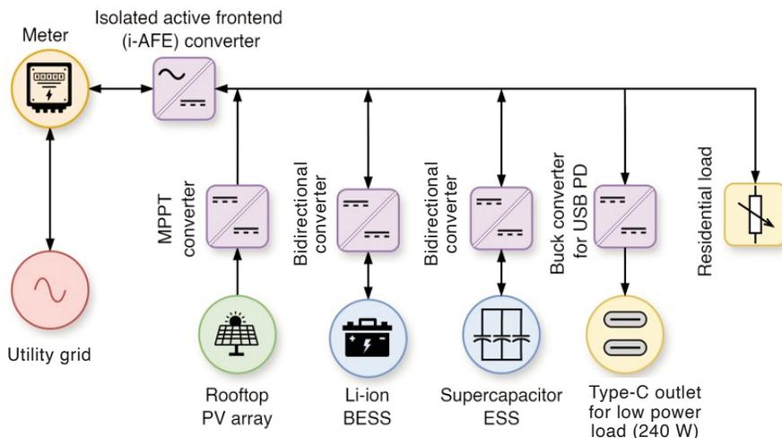
Fig. 17. Simplified schematic of a DC residential PV installation with a supercapacitor as secondary storage.
