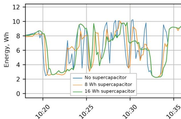
Fig. 13. Power fluctuations in the time interval 10:20–10:35 with an analysis of two proposed energy banks’ influence on the DC power flow.
