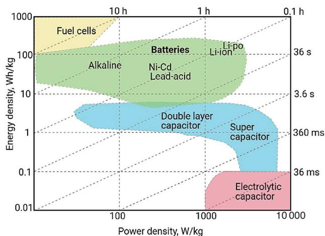
Fig. 4. Comparison of various types of energy sources by energy density and power.
