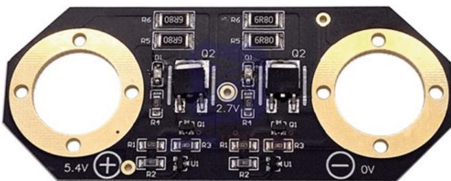
Fig. 10. Supercapacitor balancing system [32].
