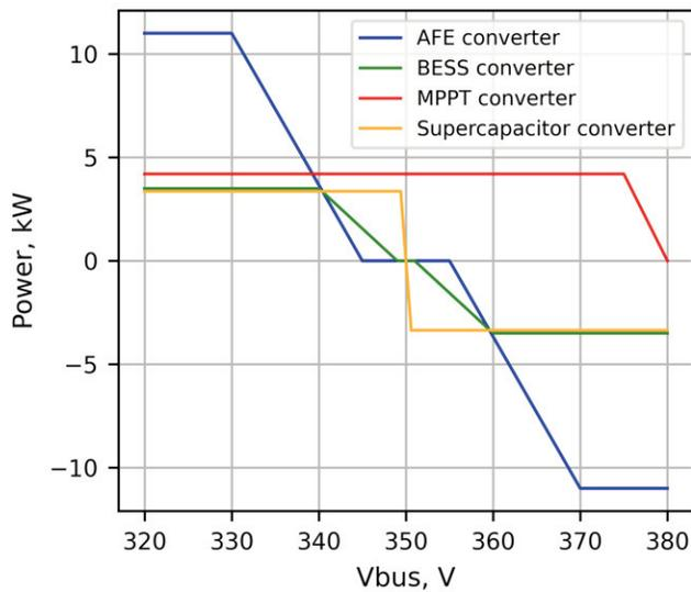
Fig. 18. Ideal droop curves of each component of the DC residential PV installation.
