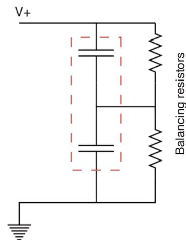
**Fig. 9.** Simplified schematic of resistor-based cell balancing.
