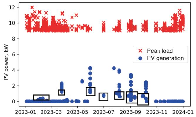
Fig. 6. Examples of PV generation dips (highlighted in black-colored boxes) during peak loads.
