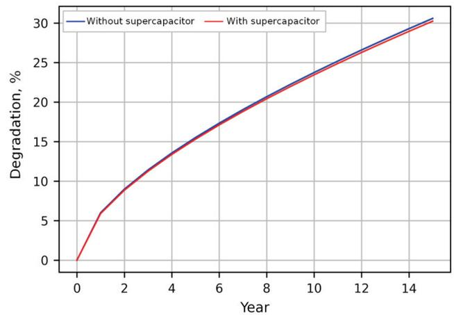
Fig. 20. Primary ESS degradation comparison for the system with and without a supercapacitor.
