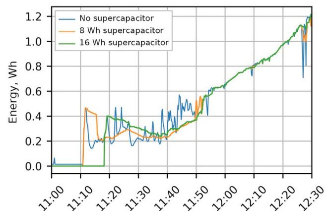
Fig. 15. Energy fluctuations in the time interval 11:00–12:30 with an analysis of two proposed energy banks’ influence on the DC power flow.
