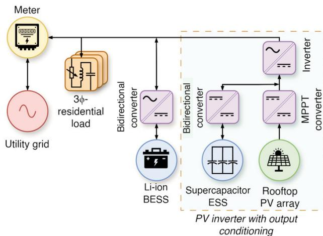
**Fig. 8.** Proposed PV microinstallation with a supercapacitor bank to stabilize generation.
