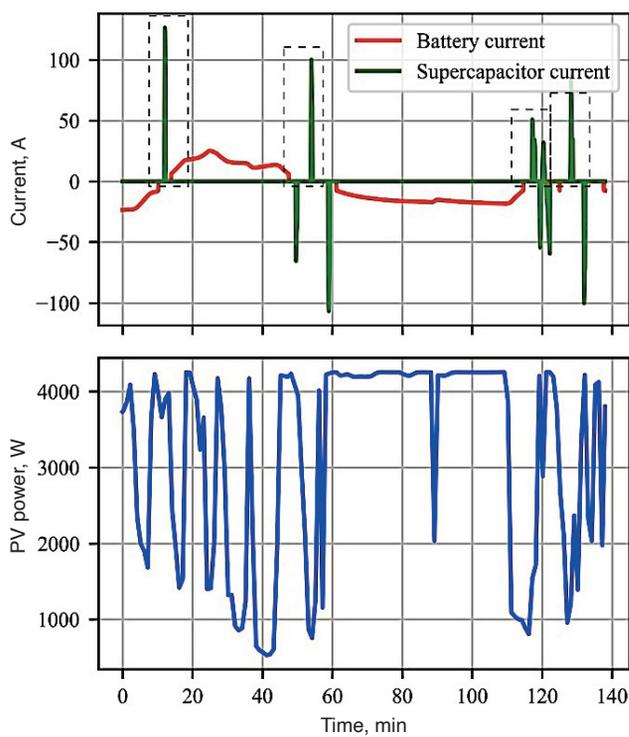
Fig. 19. Snippet of short-term PV power fluctuation mitigation through the supercapacitor in the DC microgrid. Highlighted current peaks are where PV generation dips occurred and the supercapacitor tried to stabilize the system.
