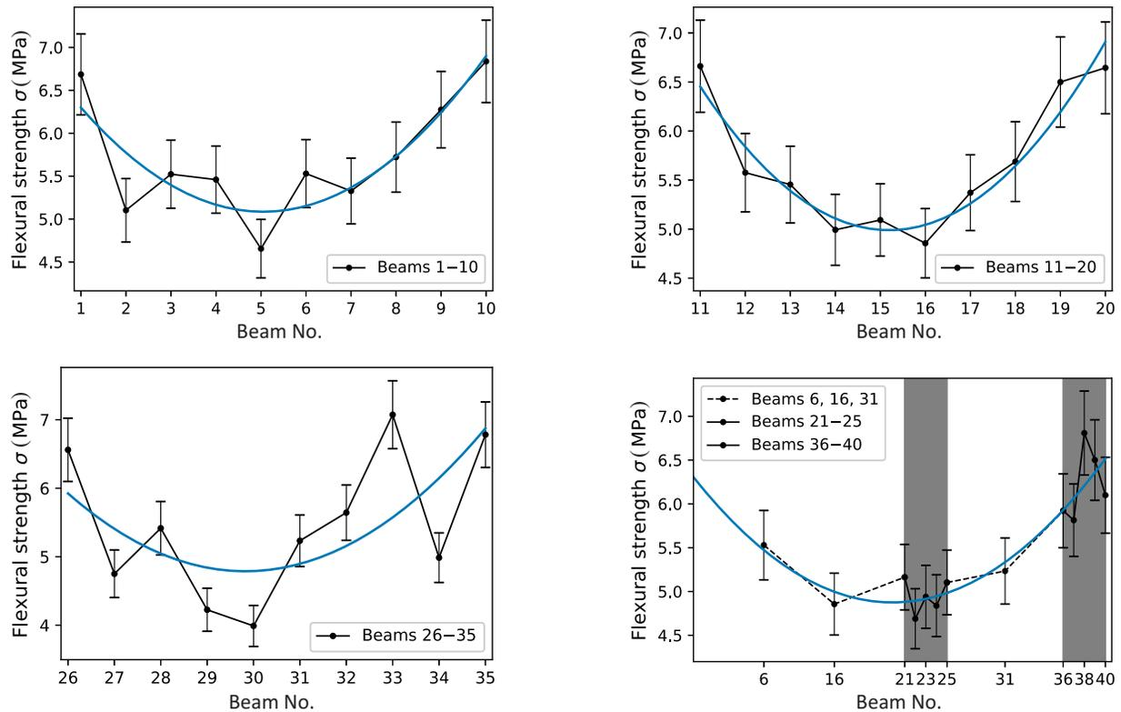
Fig. 6. Flexural strength  $\sigma$  as a function of the beam number. Least square fit graphs of the dominant trends are indicated by using the continuous lines. The lower-right plot corresponds to the centerline results highlighted in Fig. 7.
