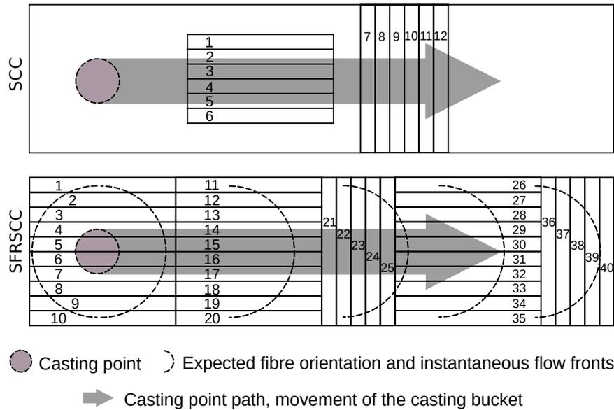
**Fig. 1.** Schematic drawing of the top view of the studied concrete slabs. Segmentation of the slab into smaller beams totalling 12 in the case of SCC and 40 in the case of SFRSCC.
