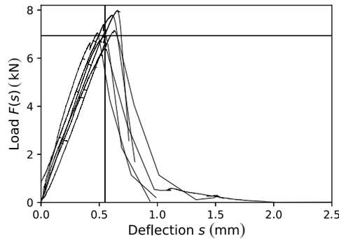
**Fig. 4.** Load history  $F(s)$  for the selected SCC beams, shown in Fig. 1. The average deflection corresponding to the main cracking  $\bar{s}_f = 0.55$  mm is depicted by the vertical line. The mean cracking load  $\bar{F}_f \equiv \bar{F}(\bar{s}_f) \approx 7.0$  kN corresponding to the selected load history graphs is indicated by the horizontal line.
