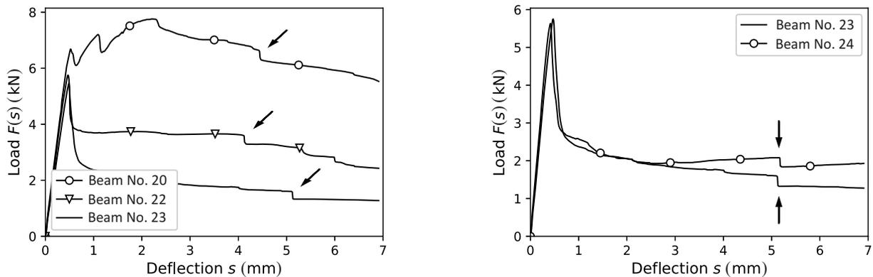
**Fig. 10.** Left: Examples of 1/3 kN events. The events are indicated by the bold arrows. Right: An example of neighbouring beams where the 1/3 kN events occurred almost precisely at the same beam deflection value  $s$ .
