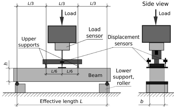
**Fig. 3.** Schematic drawing of the four-point bending test set-up, where the effective length  $L$  is 0.9 m. The zero point for the displacement is on top of a thin plate which is placed across the top of the beam in the centre, at the beginning of the test the displacement gauges are compressed.
