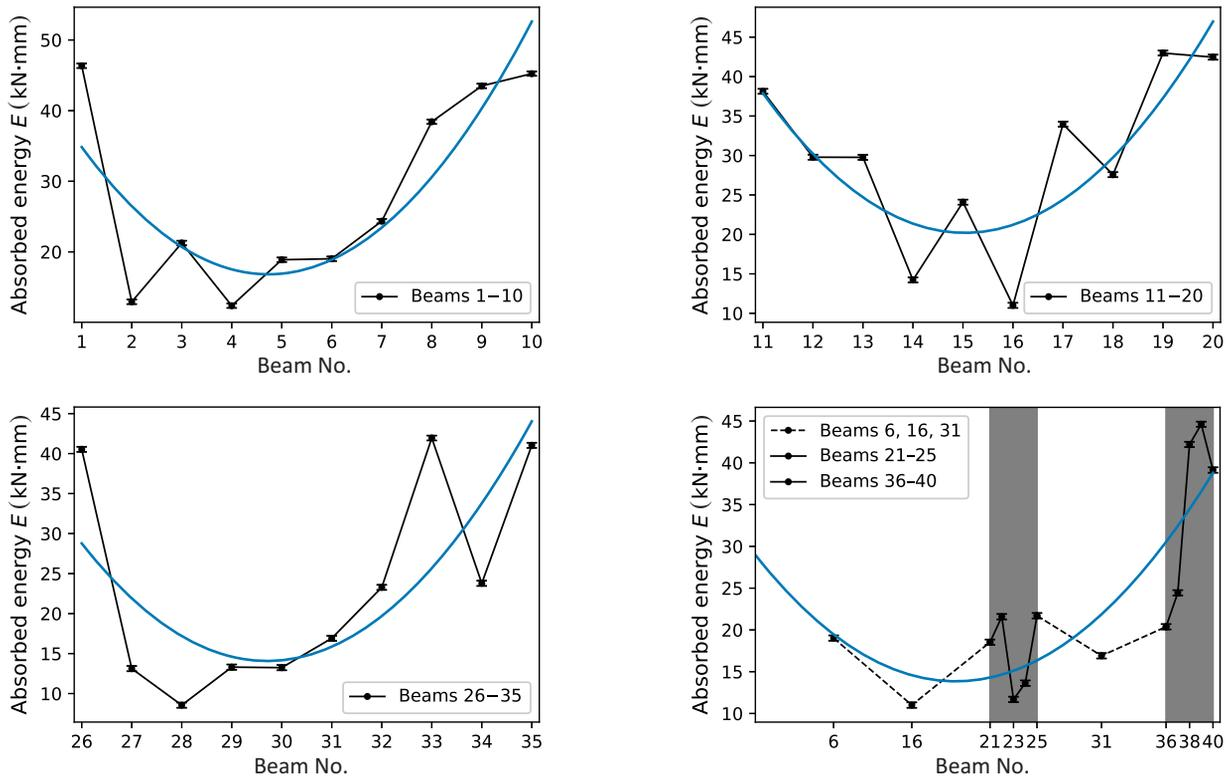
**Fig. 9.** Post-cracking absorbed energy  $E|_{s \in (s_f, s_s]}$  as a function of the beam number. Least square fit graphs of the dominant trends are indicated by the continuous lines. The lower-right plot corresponds to the centerline results highlighted in Fig. 7. The calculated uncertainty of the displayed energy values  $\delta E|_{s \in (s_f, s_s]} = \pm \xi$  kN·mm, where  $\xi \in [0.30, 0.33]$ .
