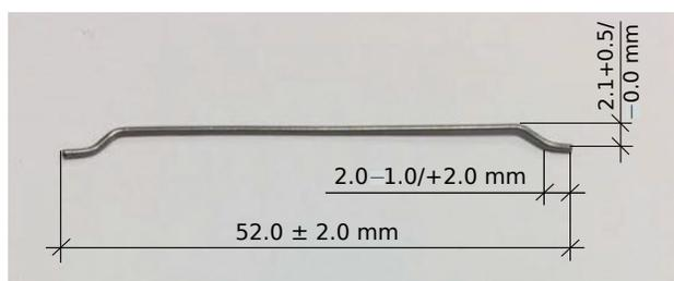
**Fig. 2.** Steel fibre used in the wet SFRSCC mix.**Table 2.** Information on the steel fibres as provided by the manufacturer [36]
