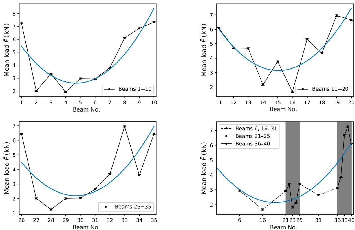
**Fig. 8.** The accepted mean post-cracking load  $\bar{F}|_{s \in (s_f, s_s)}$  as a function of the beam number. Least square fit graphs of the dominant trends are indicated by the continuous lines. The lower-right plot corresponds to the centerline results highlighted in Fig. 7. The uncertainty of the displayed accepted mean load values  $\delta \bar{F}|_{s \in (s_f, s_s)} = \pm 50$  N.
