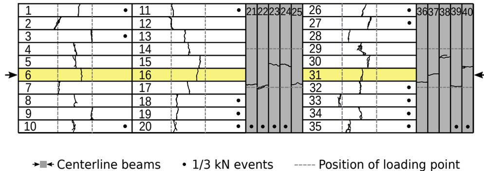
Fig. 7. Centerline beams numbered 6, 16, 21–25, 31, 36–40 are highlighted by the coloured backgrounds and bold arrows. The positions and shapes (bottom view) of the cracks sustained at the main cracking are shown based on the realistic crack patterns.
