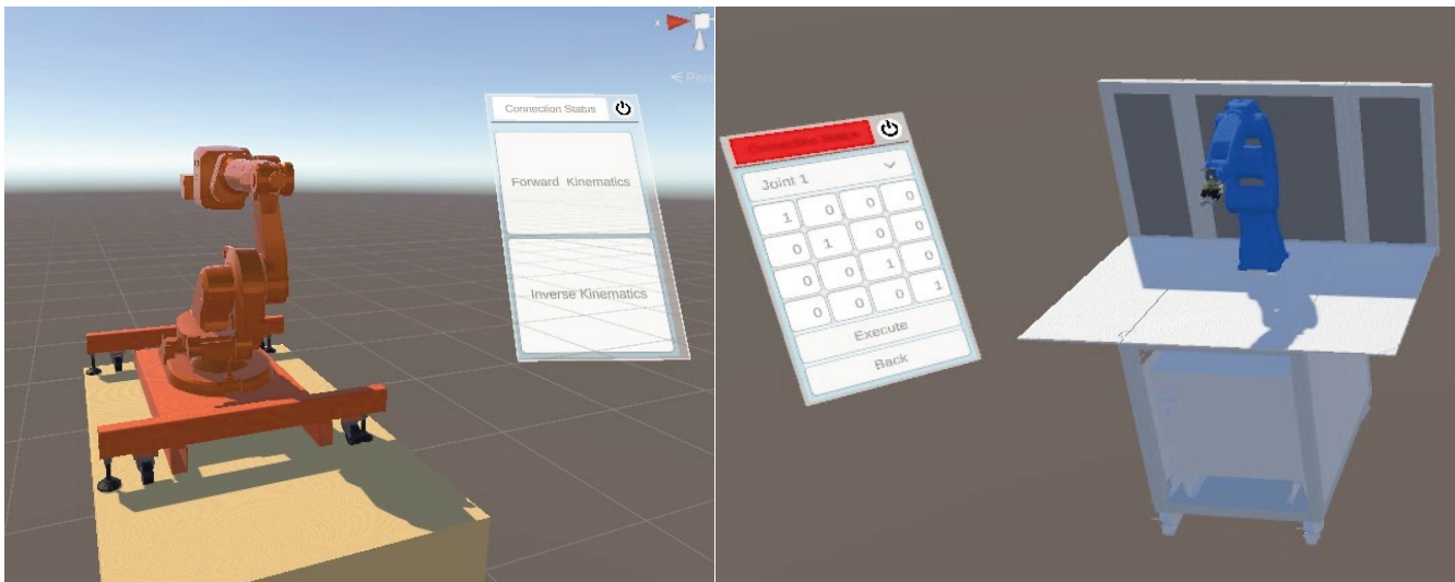
Fig. 6. ABB IRB 1600 and Yaskawa Motoman GP8 digital twins and interactive kinematics application prototype.
