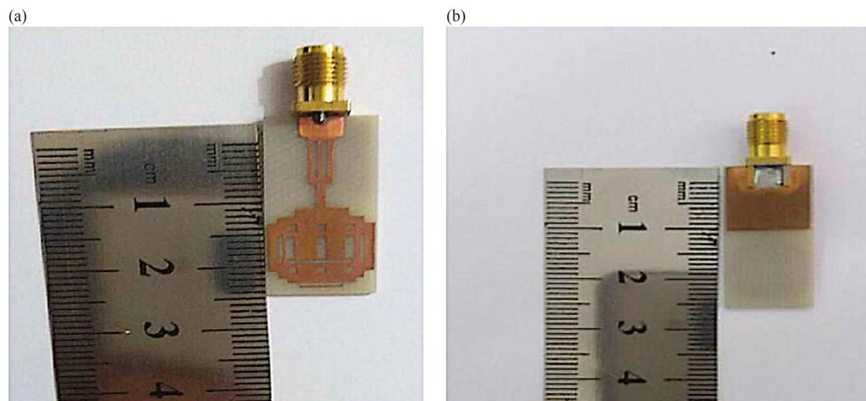
Fig. 10. The prototype of the designed UWB antenna: top view (a) and bottom view (b).
