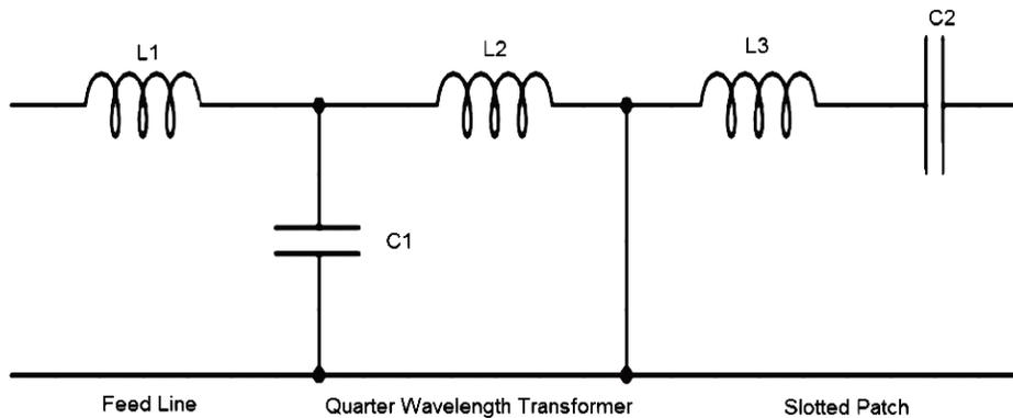
Fig. 4. The circuit equivalent of the projected antenna.
