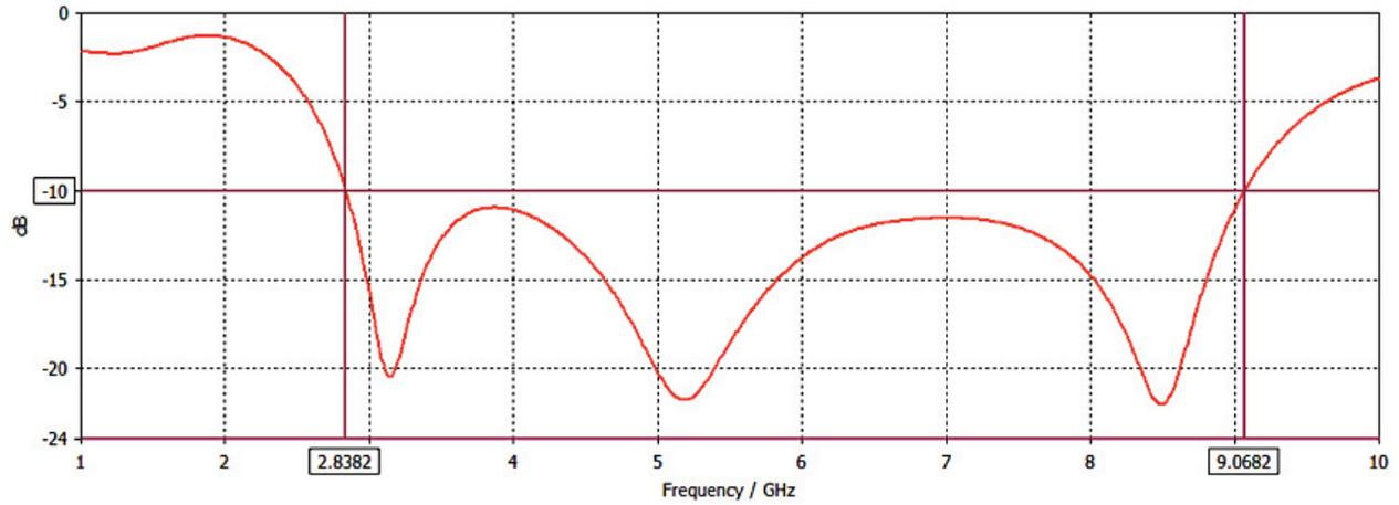
Fig. 5. Input reflection for the simulated antenna.
