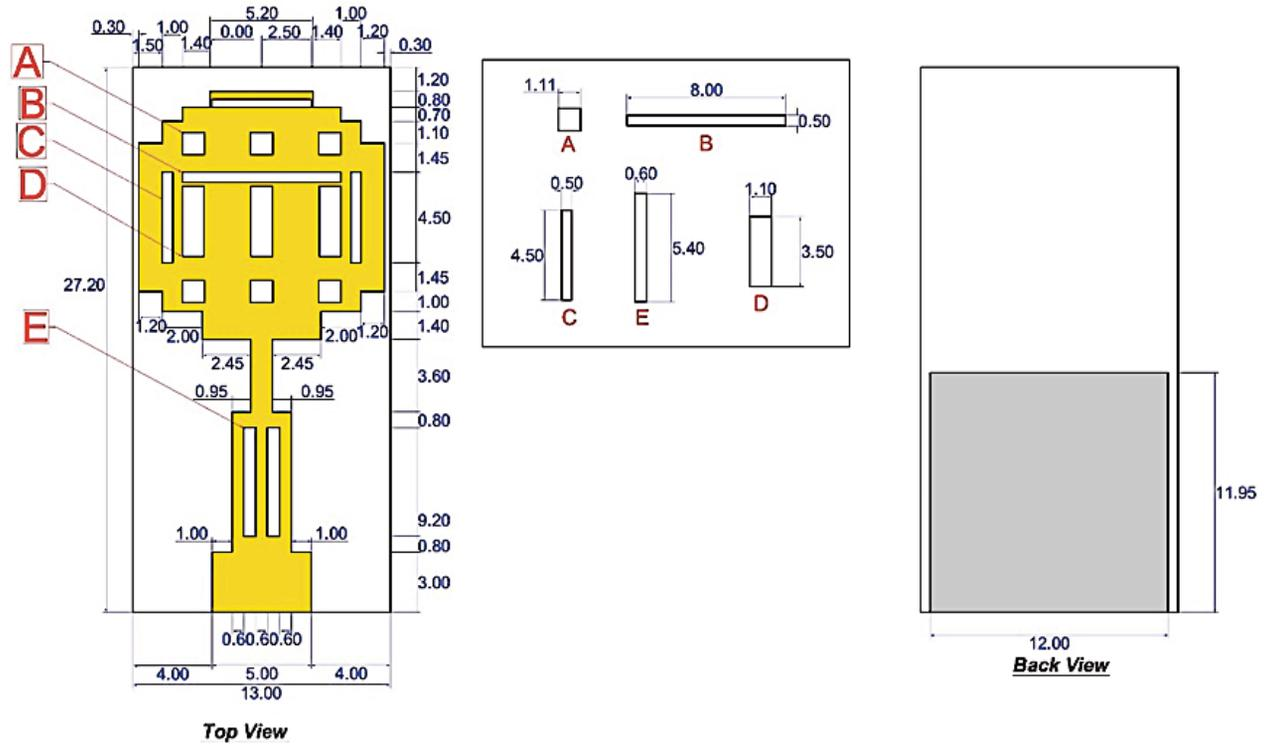
Fig. 3. The geometry for the projected antenna.
