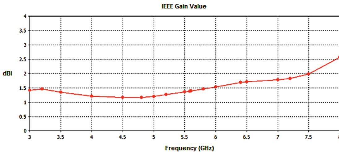
Fig. 8. Gain result for the projected antenna.
