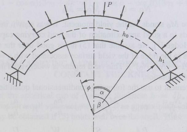
Fig. 1. Shell geometry.
