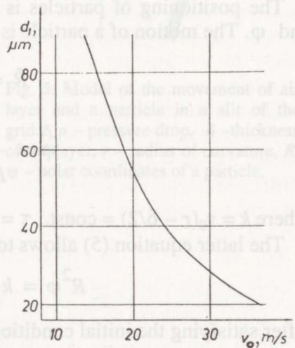
Fig. 8. Dependence of the size of bound particle  $d_1$  of classification on the air velocity  $v_0$  in the classifier.
