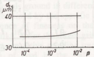
Fig. 11. Dependence of the size of bound particle on voluminal concentration of particles in the air. The ordinary concentration is less than  $\beta < 10^{-3}$ .
