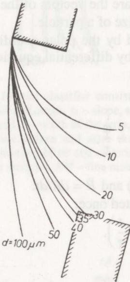
Fig. 7. Movement of coal particles of various size in a slit of the grid. In these conditions the size of bound particle is  $33 \mu\text{m}$ .
