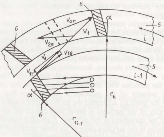
Fig. 2. Particle movement between and in the treatment rings 5. A particle falls on the grinding tools (blade) 6, breaks, slides along the blade and leaves it with velocity  $v_1$ . The velocity of next collision is  $v_{0r}$ .
