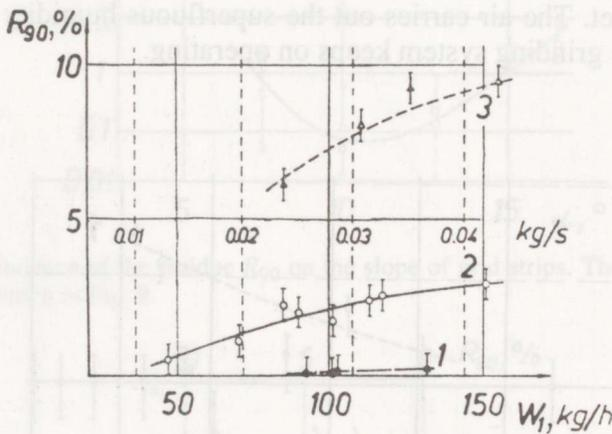
Fig. 15. Dependence of  $R_{90}$  on the productivity of disintegrator for different air aspiration through the grid: 1 -  $Q_{asp} = 0.125Q_{am}$ , 2 -  $Q_{asp} = 0.25Q_{am}$ , 3 -  $Q_{asp} = Q_{am}$ .
