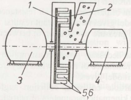
Fig. 1. A disintegrator consists of two rotors 1, 2 and two motors 3, 4 revolving in opposite directions. Each rotor contains one or more treatment rings 5, they consist of a number of grinding tools 6.
