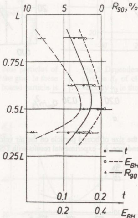
Fig. 13. Variability of the quality of classification along the longitude of the grid.  $t$  - parameter of sharpness of separation,  $E_{BH}$  - Barski-Hancock coefficient,  $R_{90}$  - residue on the sieve with the meshes of  $90 \mu\text{m}$ .
