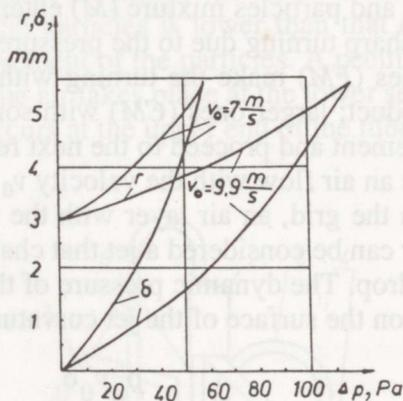
Fig. 6. Dependence of the air layer thickness  $\delta$  and that of the curvature radius  $r$ , on the pressure drop in the grid.
