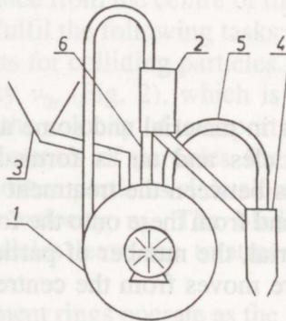
Fig. 3. Disintegrator under the separative grinding conditions. 1 – Disintegrator, 2 – Classifier, 3 – Material feeder, 4 – Separation of fine particles from air, 5 – Air circulation, 6 – Coarse material circulation.
