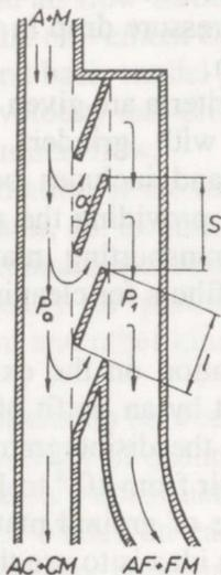
Fig. 4. Inertial classifier consists of a grid of sloped strips.  $\alpha$  – slope,  $s$  – step of the grid,  $l$  – width of the strip,  $p_0$ ,  $p_1$  – pressure before and after the grid,  $A+M$  – mixture of air and material,  $CM$  – coarse material,  $FM$  – fine material.
