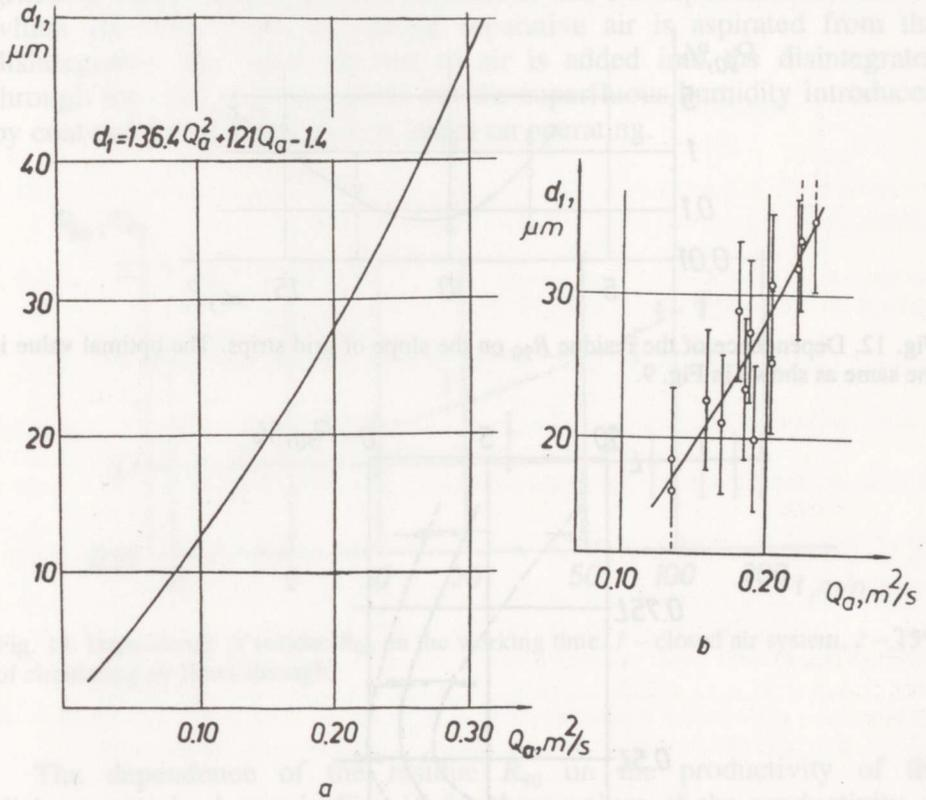
Fig. 10. Dependence of the size of bound particle on the air velocity in the grid slit for coal: *a* – theoretical dependence; *b* – experimental results with DSL-38.
