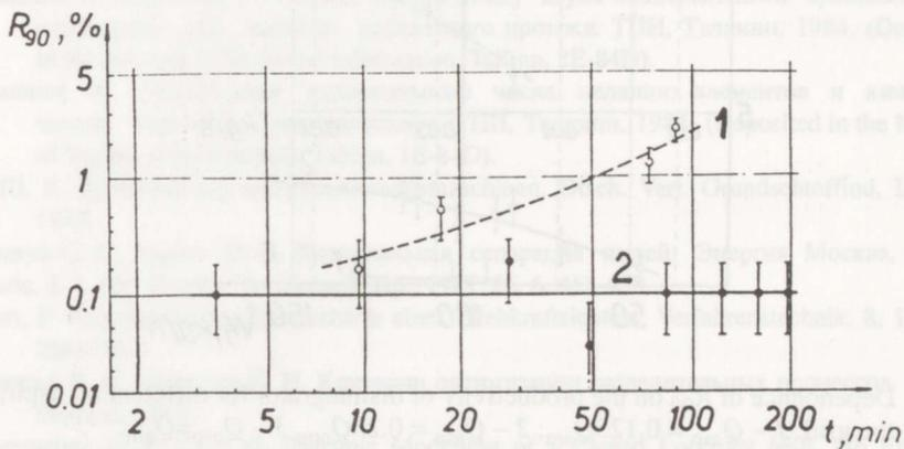
Fig. 14. Dependence of residue  $R_{90}$  on the working time. 1 – closed air system, 2 – 15% of circulating air flows through.
