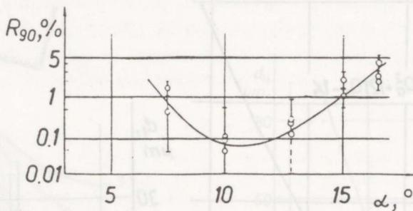
Fig. 12. Dependence of the residue  $R_{90}$  on the slope of grid strips. The optimal value is the same as shown in Fig. 9.
