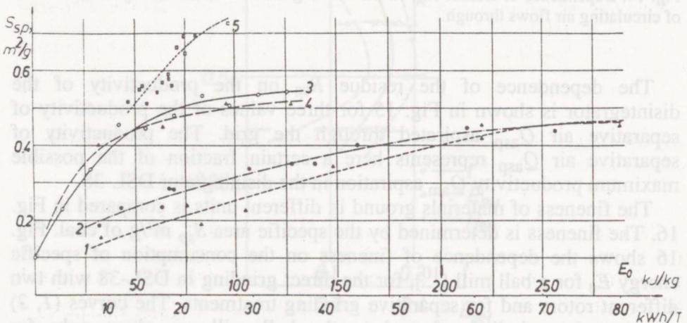
Fig. 16. Dependence of specific surface area  $S_{sp}$  on the specific energy consumption  $E_0$ : 1, 2 - a ball mill [4], 3, 4 - DSL-38 direct grinding with three and five row rotors, correspondingly, 5 - DSL-38 under the condition of separative grinding.
