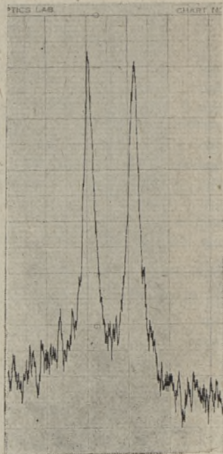
Fig. 3. C^{13} absorption spectrum of benzene (2 ml). Sweep rate 6.25 cps/sec.
