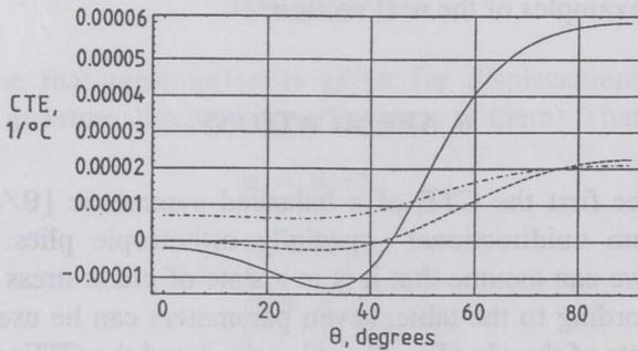
Fig. 3. Longitudinal coefficient of thermal expansion (CTE) as a function of ply angle for three  $[\theta/-\theta]_{ns}$  laminates consisting of different commercial ply materials: Kevlar-epoxy (solid line), graphite-epoxy (dashed line), and E-glass-epoxy (dash-dot line).
