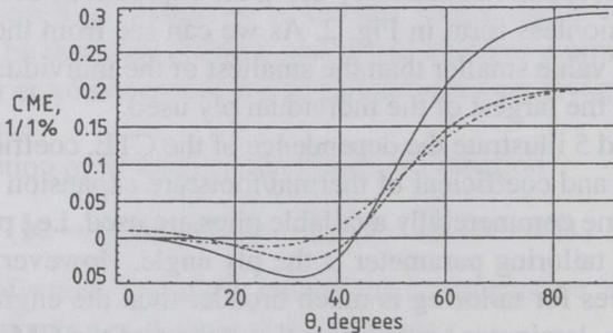
Fig. 4. Longitudinal coefficient of moisture expansion (CME) as a function of ply angle for three  $[\theta/-\theta]_{ns}$  laminates consisting of different ply materials: Kevlar-epoxy (solid line), graphite-epoxy (dashed line), and E-glass-epoxy (dash-dot line).
