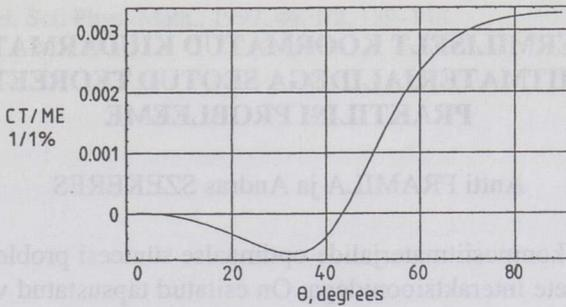
Fig. 5. Longitudinal coefficient of thermal/moisture expansion (CT/ME) as a function of ply angle for a  $[\theta/-\theta]_{ns}$  graphite-epoxy laminate.
