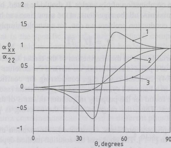
Fig. 2. Dimensionless longitudinal coefficient of thermal expansion of a  $[\theta/-\theta]_{ns}$  laminate as a function of ply angle. Ply properties:  $E_{11}/E_{22} = 10$ ,  $\nu_{12} = 0.25$ ,  $\alpha_{11}/\alpha_{22} = 0.1$ ;  $G_{12}/E_{22} = 0.05, 0.5$ , and 4 for curves 1, 2, and 3, respectively.
