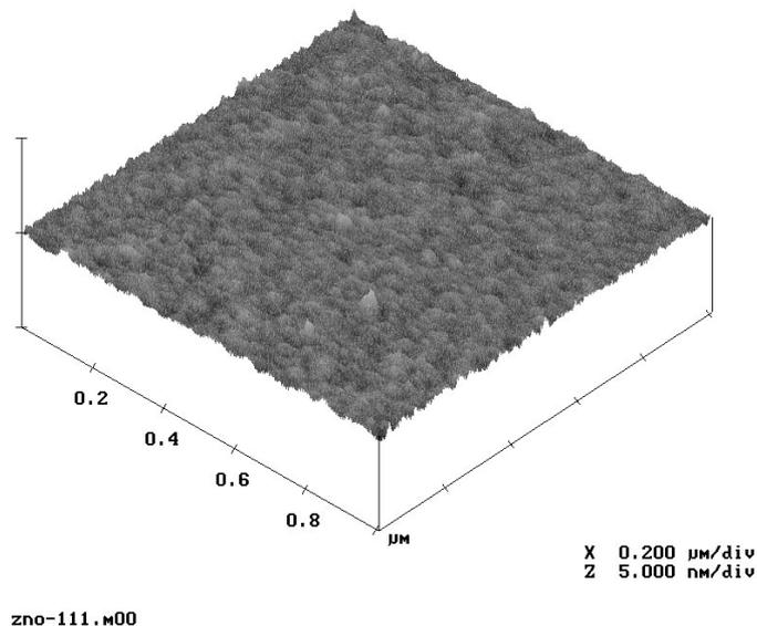
**Fig. 4.** Atomic force microscopy image of ZnO film obtained by atomic layer deposition using a single exchange chemical reaction on (1 1 1) silicon substrate.
