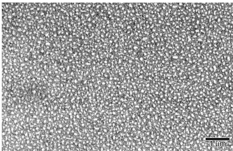
**Fig. 7.** Scanning electron microscopy image of a relatively large area of the ZnO/Ag/Si (1 1 1) film taken at room temperature.
