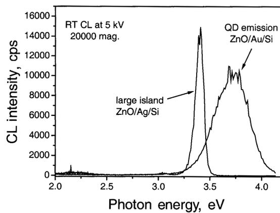
**Fig. 6.** Spot-mode cathodoluminescence (CL) spectra of two ZnO samples grown on (1 1 1) silicon covered with Ag or Au thin layers. Emission of CL from a large island, observed in the ZnO/Ag/Si sample, and from quantum dot (QD) objects in ZnO/Au/Si is shown.
