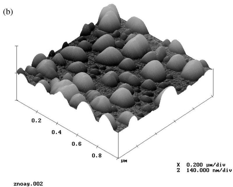
**Fig. 8.** Atomic force microscopy images of ZnO dot-like structures grown by atomic layer deposition using a single exchange chemical reaction on (1 1 1) silicon substrate covered with a thin layer of Au (a) and Ag (b).
