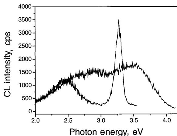
**Fig. 3.** Room temperature cathodoluminescence (CL) of two ZnO films grown by atomic layer deposition using single exchange chemical reaction. Sharp excitonic “edge” CL is observed for the film grown on ZnS/(1 1 1) Si. We also show broad and weak CL of the ZnO/GaAs film showing a rough surface and three-dimensional growth mode.
