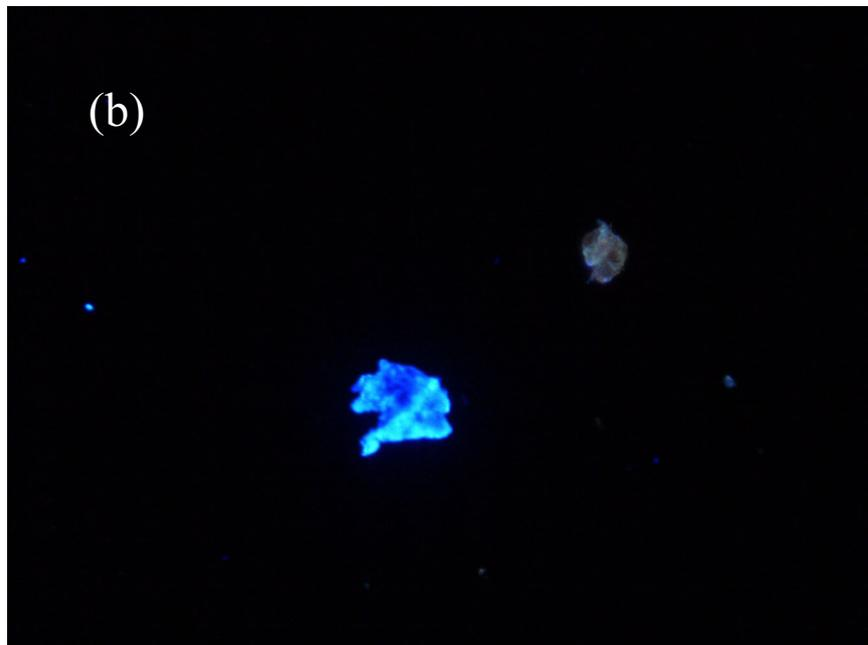
**Fig. 5.** Micro-photoluminescence (PL) images of the thin ZnO layer grown by atomic layer deposition using a single exchange chemical reaction. Image (a) was taken with a blue low pass filter, (b) with a UV low pass filter. The “edge” PL of ZnO is observed only from larger islands.
