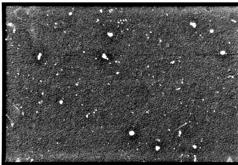
**Fig. 2.** Micro-photoluminescence image taken with Nomarski microscope showing surface morphology of an oxidized ZnS film. The ZnS film was grown by atomic layer deposition on (1 1 1) silicon substrate using a double exchange chemical reaction and was post-growth annealed in oxygen flux.
