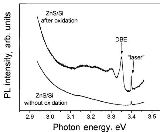
**Fig. 1.** Low-temperature photoluminescence (PL) spectra of the ZnS film grown by atomic layer deposition on silicon, taken before and after oxidation. The upper curve, taken after annealing the sample at a temperature of 550 °C, shows the appearance of ZnO “edge” emission of excitonic origin, attributed by us to radiative recombination of donor bound excitons (DBE).
