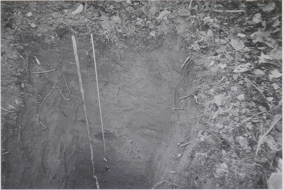
Photo 2. Profile No. 4 of Chromi-Stagnic Luvisol (A–Baf–ELg–Bt) on the drumlin slope in 1994. Photo by Toomas Frey.
