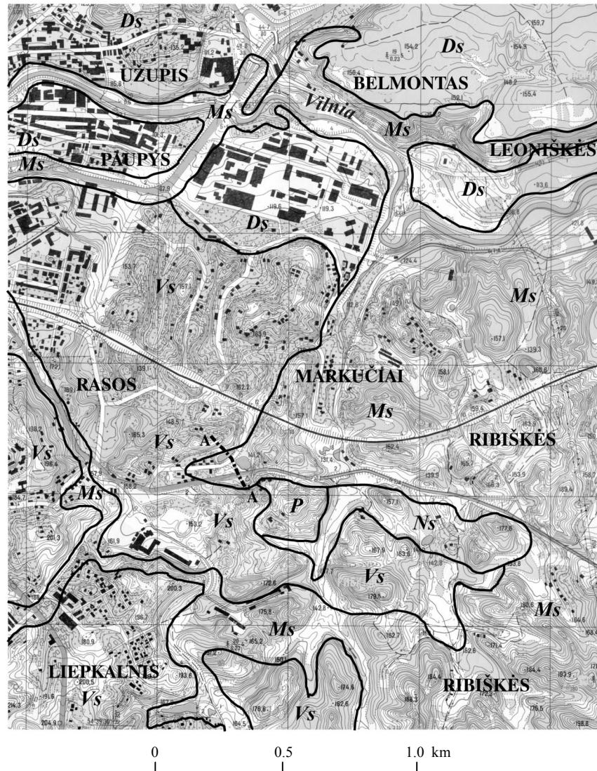
Fig. 3. The slope stability areas of Rasos–Ribiškės erosional hills: Ns, unstability; Ms, low stability; Vs, medium stability; P, stability; Ds, high stability; A–A, levelling profile.
