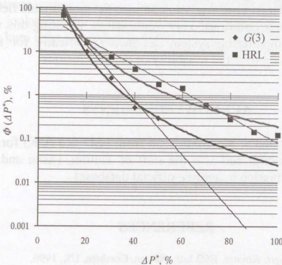
**Fig. 5.** Frequency of occurrence of wind power increments for the group of three  $G(3)$ ; — power function, - - exponential function.
