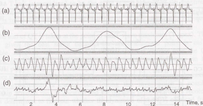
Fig. 3. A fragment of recorded signals: (a) ECG; (b) ventilation impedance; (c) heart impedance; (d) signal from the piezoelectric transducer.
