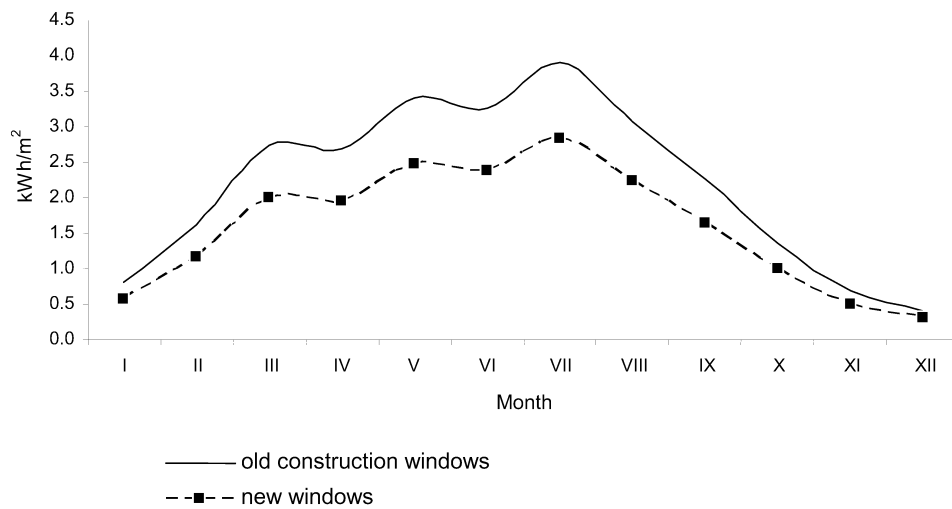
Fig. 5. Heat inflow of solar radiation through existing and changed windows.
