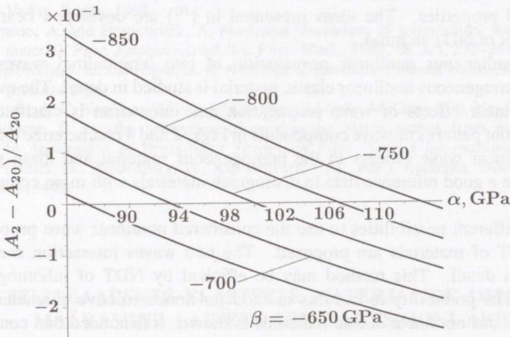
Fig. 7. Second harmonics relative amplitude versus material elasticity parameters.
