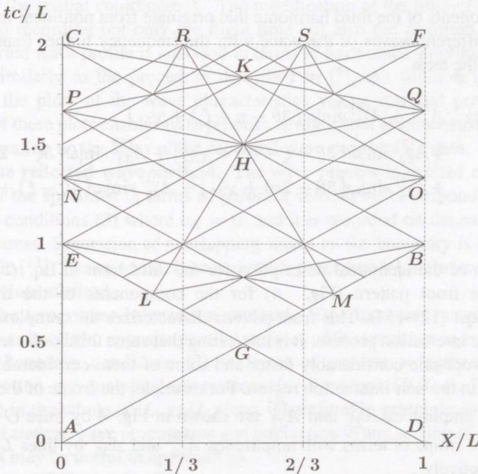
Fig. 4. Front pattern of the wave components. Third order small terms in Eq. (5).
