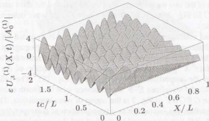
**Fig. 1.** Longitudinal wave interaction in a homogeneous nonlinear elastic material,  $A_0^{(1)} \equiv \varepsilon a_0$ .
