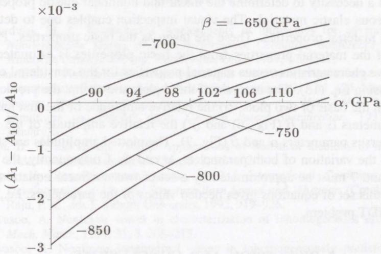
Fig. 6. First harmonics relative amplitude response to the variation of linear and nonlinear elastic properties of the material.
