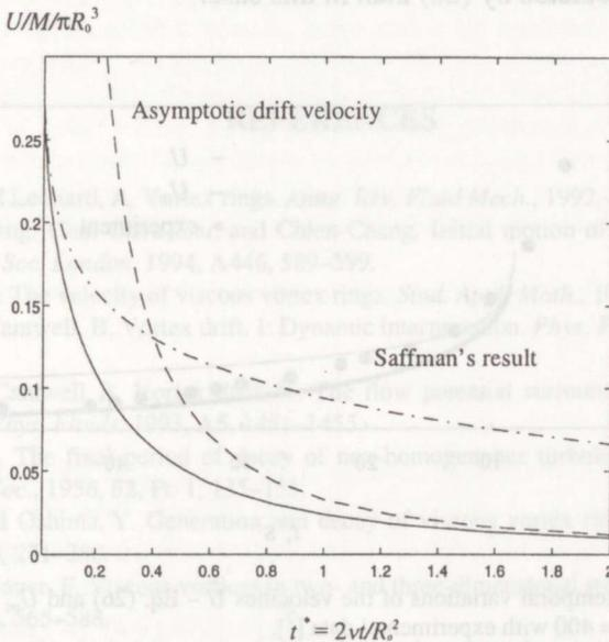
Fig. 3. Time variation of the translation velocity of a viscous vortex ring (solid line). Dashed line shows the asymptotic drift velocity and the dashdot line is the result from [3].
