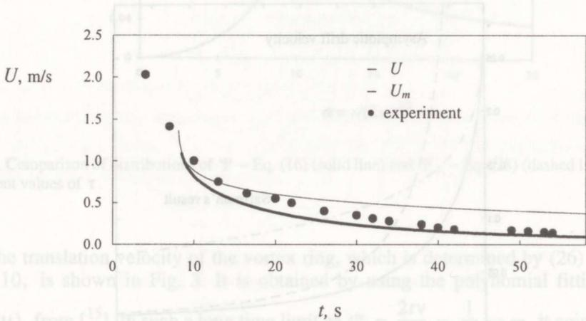
Fig. 4. Comparison of temporal variations of the velocities  $U$  – Eq. (26) and  $U_m$  – Eq. (29) for the Reynolds number  $\text{Re}_0 = 400$  with experimental data [7].
