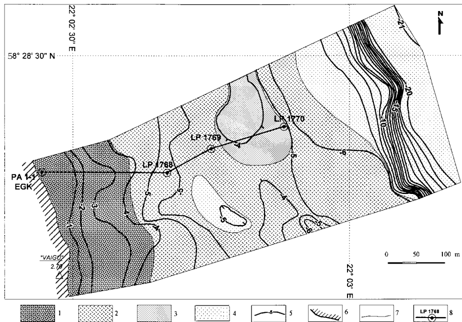
Fig. 15. Bottom deposits at the Vaigu harbour site (from [1], modified): 1 – gravel with pebbles and cobbles; 2 – mixed sand; 3 – medium sand; 4 – fine sand; 5 – bathymetric isoline; 6 – average waterline; 7 – margins between sediment types; 8 – cross-section line, with investigation points and their numbers (see Fig. 17).
