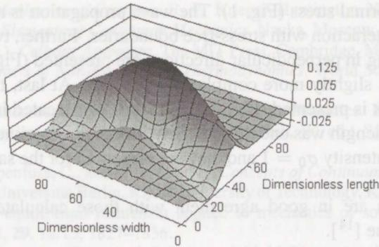
**Fig. 1.** Surface plot of the distribution of the normal stress in a rectangular specimen excited at the left boundary.
