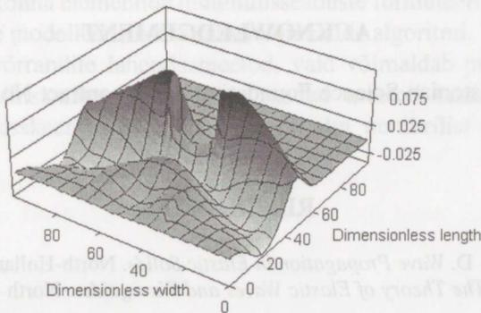
**Fig. 3.** Surface plot of the distribution of the normal stress in the case of interaction of the elastic wave with a crack in the middle of the specimen.
