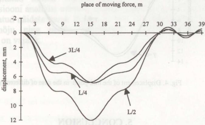
Fig. 2. Displacement at points  $L/4$ ,  $L/2$ ,  $3L/4$  of the examined structure.
