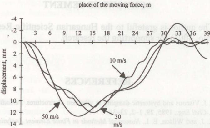
Fig. 3. Displacement of the mid-point at different velocities.
