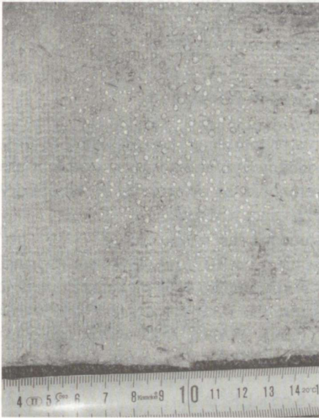
Fig. 3. Photo of condensation on the internal surface of the wood fibreboard specimen No. 2 at t = 276 \text{ h} .
