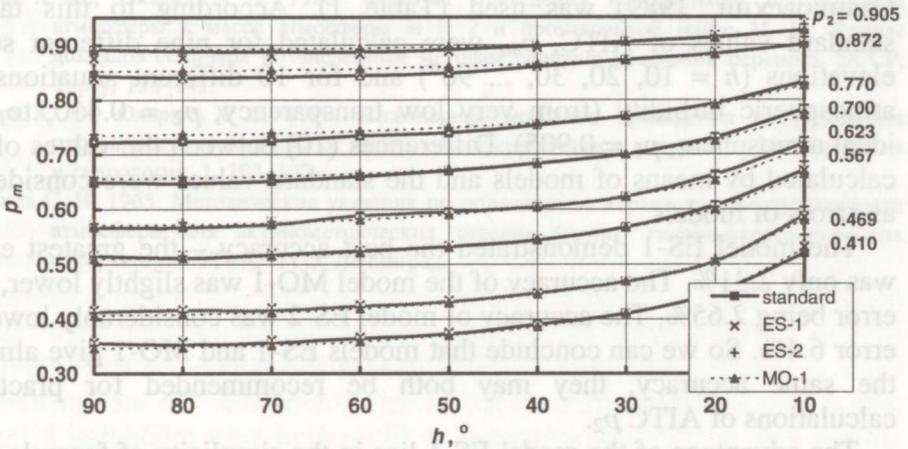
Fig. 2. Values of AITC  $p_m$  as functions of diminishing solar elevation angle,  $h$ .
