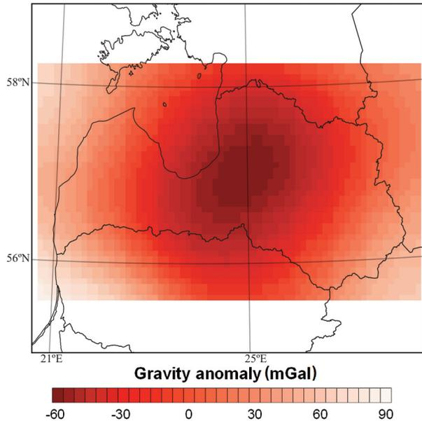
**Fig. 6.** Modelled gravity response of the European Moho map (Grad et al. 2009). The amplitude of the negative anomaly in the territory of Latvia reaches 142 mGal.
