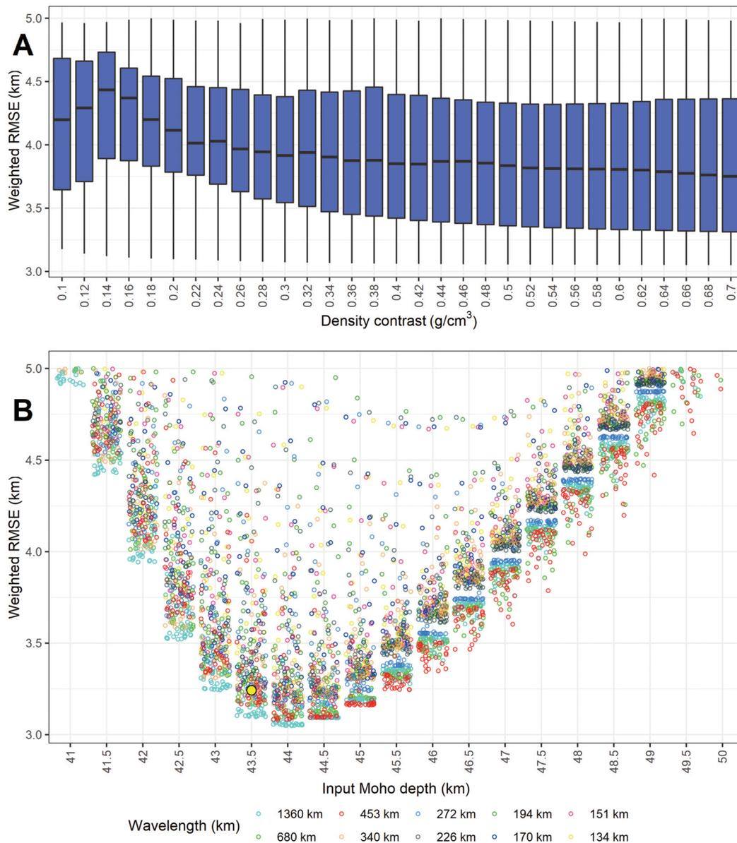
**Fig. 5.** Weighted RMSE in relation to modelling parameters. **A**, density contrast; **B**, filter wavelength and input depth. The large yellow dot marks the selected model. All models with weighted RSME  $\geq 5$  km are not shown.
