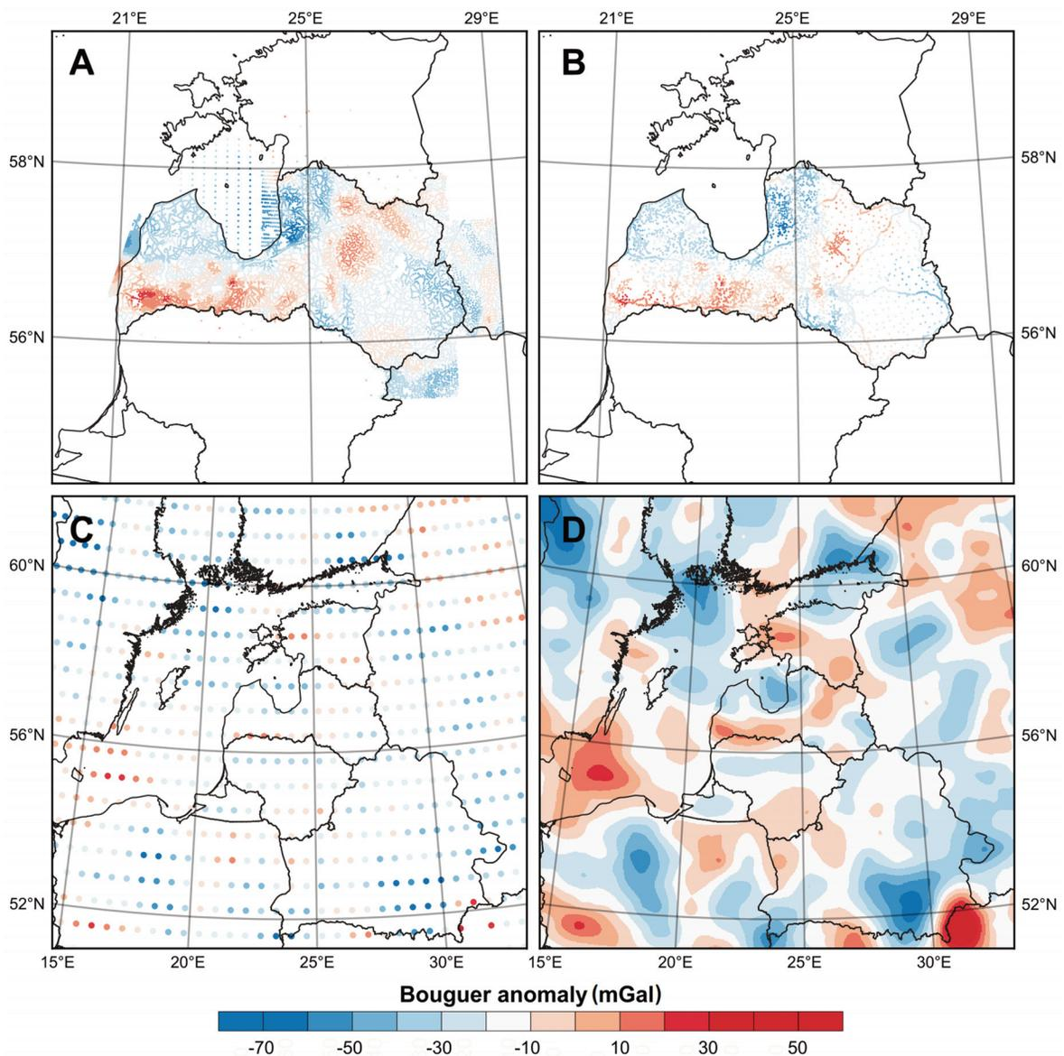
**Fig. 2.** Overview of gravity measurements in Latvia. **A**, dots represent calculated Bouguer anomaly from the geophysical mapping measurements from of the USSR-era (Kaminskis 2010); **B**, Bouguer anomaly from the gravity measurements by the Geodetic Survey of Latvia (Zandersons et al. 2018); **C**, Bouguer anomaly sampled from the EIGEN-6S4 satellite model (Förste et al. 2016); **D**, gridded and combined gravity data.
