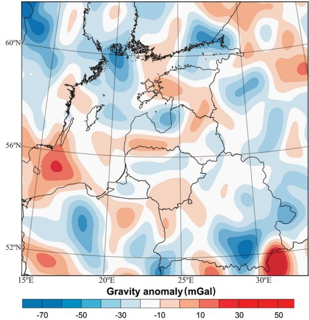
**Fig. 3.** The low-pass filtered gravity data of Fig. 2D, used in the calculation of the best performing model. The filter cut-off wavelength is 134 km.
