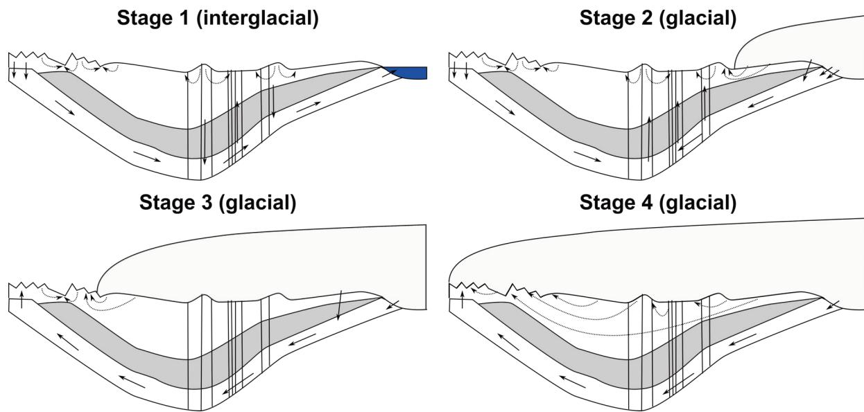
**Fig. 2.** Presumed flow patterns in interglacial and glacial periods, controlled by the expansion and retreat of the ice sheet. In the shallow aquifers (dashed arrows) and the Liepaja–Pskov fault zone, flow is mainly driven by topography during interglacial periods (Stage 1). During glacial periods (Stages 2–4), it is assumed that the fault zone has negligible influence on water flows and flow is mainly driven by ice sheet topography (Gerber et al. 2017). From Gerber et al. (2017).
