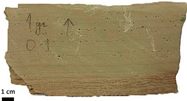
Fig. 3. Irregularly laminated dolomite from the Dārzciems dolomite quarry (layer 1, facie F1).
