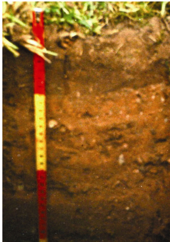
Fig. 2. Calcaric Cambisol profiles under grass-herbaceous sward in 1984 (a), 1994 (b), and 2004 (c) when the layer between 10 and 20(30) cm had dried to the discontinuous capillary moisture level, which caused the compactness and a lighter value of chroma there.
