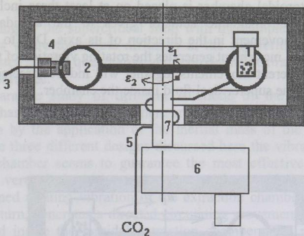
Fig. 2. Scheme of a toroidal extraction chamber. 1, sample in a porous cartridge; 2, extraction chamber; 3, restrictor; 4, valve; 5, capillary; 6, mechanical actuator; 7, shaft.
