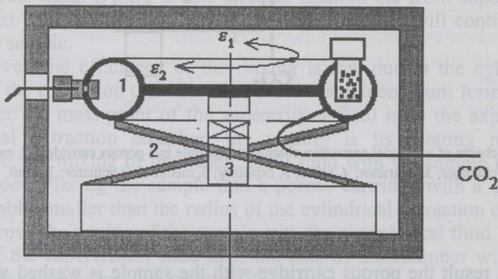
Fig. 3. Scheme of a vibrating toroidal extraction chamber. 1, toroidal chamber; 2, spring rods; 3, electromagnetic actuator.
