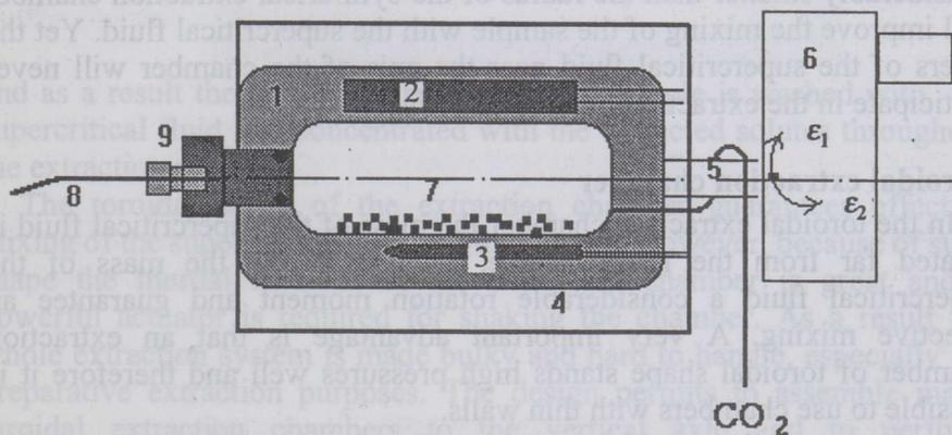
Fig. 1. Scheme of a cylindrical extraction chamber. 1, stainless steel body; 2, heating element; 3, thermosensor; 4, thermal insulating material; 5, axle; 6, shaking mechanism; 7, sample; 8, restrictor; 9, valve.
