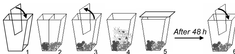
Fig. 1. Scheme of the test procedures: (1) Introduction of the movable wall in the centre of the test vessel; (2) Introduction of the soils to be tested in each side (control versus spiked soil); (3) Movable wall is removed; (4) Introduction of ten enchytraeid worms in the centre of the vessel; (5) Covering the test vessel with a lid (perforated); 48 hours period (16:8 h light:dark; 20 \pm 2^\circ\text{C} ); (6) Re-introduction of the wall to separate the soils and counting of the organisms present in each side.
