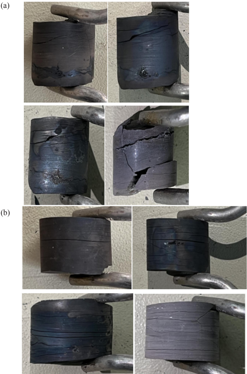
Fig. 4. Core fracture propagation networks and structural failure conditions highlighting: (a) horizontal bedding expansion, and (b) vertical bedding fracture intersections.
