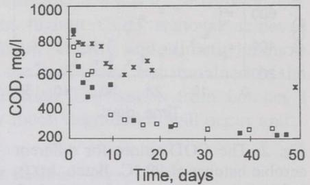
Fig. 5. The COD values for the intermittently aerated batches at 29 °C. Batch 15, 1 day aerobic, 6 days anaerobic (■); batch 16, 1 day aerobic, 6 days anaerobic (□); batch 19 6 hours aerobic, 7 days anaerobic (\*)
