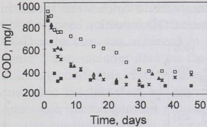
Fig. 2. The COD values for different aerobic batches at 29 °C. Batch 1 ( $\square$ ); batch 3, nutrients ( $\blacktriangle$ ); batch 5, inoculum ( $*$ ); batch 11, nutrients, inoculum ( $\blacksquare$ )
