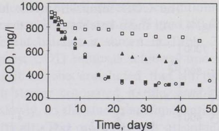
Fig. 3. The COD values for different anaerobic batches. Batch 2, 29 °C ( $\square$ ); batch 4, 29 °C, nutrients ( $\blacktriangle$ ); batch 7, 29 °C, inoculum ( $\blacksquare$ ); batch 9, 12 °C, nutrients, inoculum ( $\circ$ )
