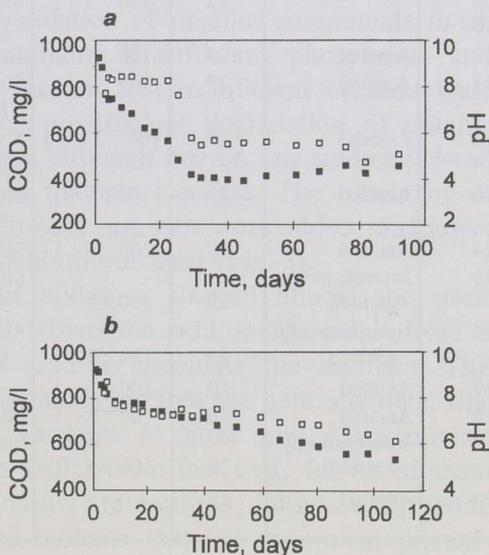
Fig. 1. Changes of the COD (■) and pH (□) values with time in aerobic batch 1 (A) and anaerobic batch 2 (B) when nothing was added to the leachate in batches
