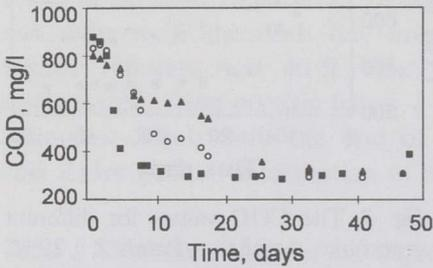
Fig. 4. The COD values for aerobic batches at 10-12 °C. Batch 6, 12 °C, nutrients, inoculum (■); batch 17, 10 °C, nutrients (▲); batch 18, 10 °C, nutrients, inoculum (○)
