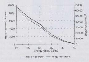
A revision has been made of oil shale reserves according to market economy conditions (Fig. 8). The bases for the prognosis is the electricity demand projection and presumption the that utilisation energy per gross domestic product decrease must signifi-One takes the cantly. 35 rating of energy
