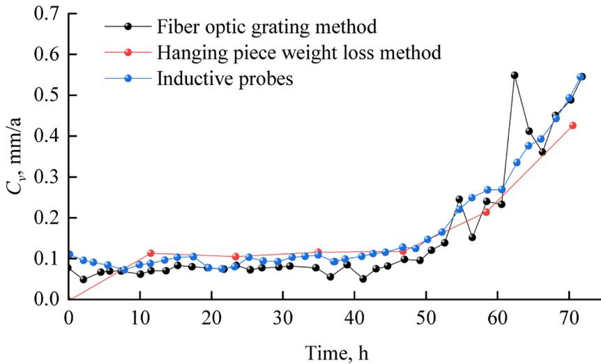
Fig. 8. Comparison of corrosion rates of different monitoring methods.
