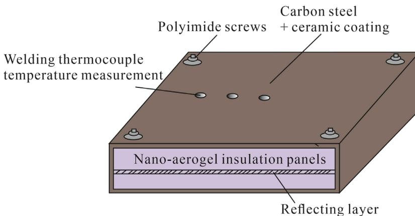
**Fig. 10.** Test system insulation.
