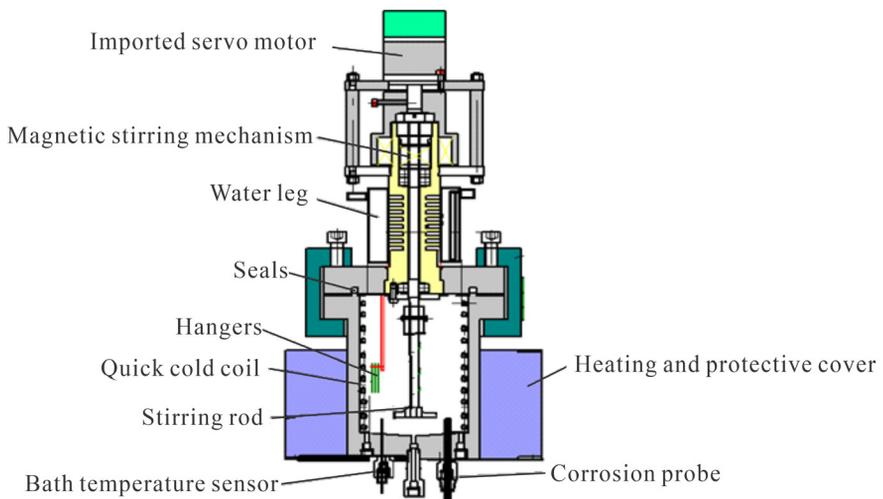
**Fig. 4.** Structure of high-temperature reaction kettle.
