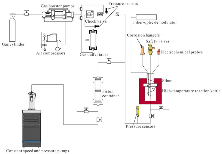
**Fig. 3.** Schematic diagram of corrosion system.
