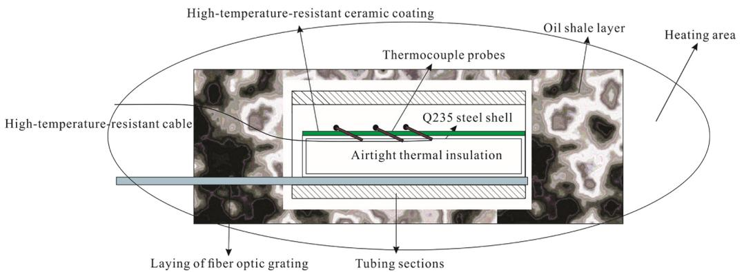
**Fig. 9.** Schematic diagram of the structure of the lower entry short section.
