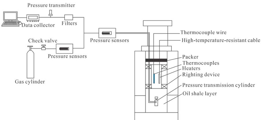
**Fig. 2.** Schematic diagram of temperature measurement system.
