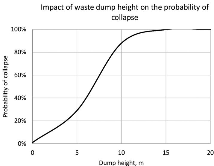
Fig. 5. Impact of the waste dump height on the probability of rooms collapse (illustrative).
