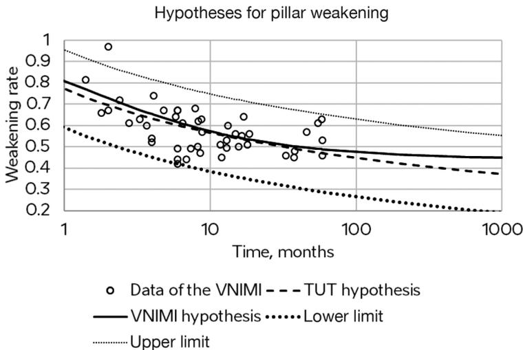
Fig. 4. Two hypotheses for the weakening of pillars as a result of oil shale creep.
