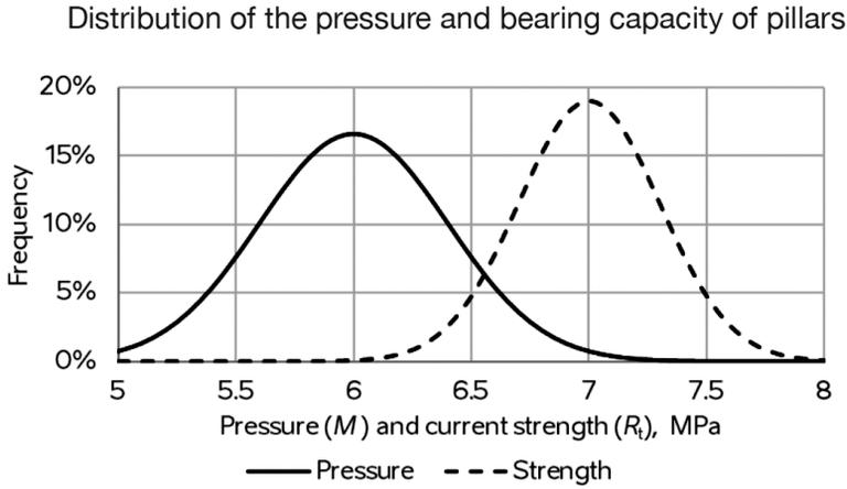
Fig. 3. Distribution of pressure in pillars and their strength (illustrative).
