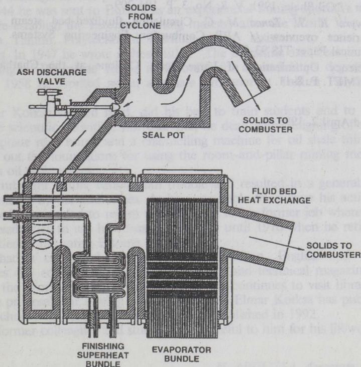
**Fig. 2. Seal pot, ash discharge valve and fluid bed heat exchanger**
