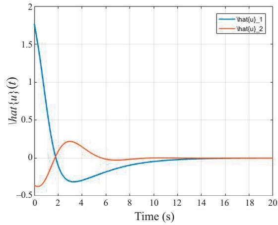
**Fig. 3.** Control input  $\hat{u}$  during stabilization maneuver.
