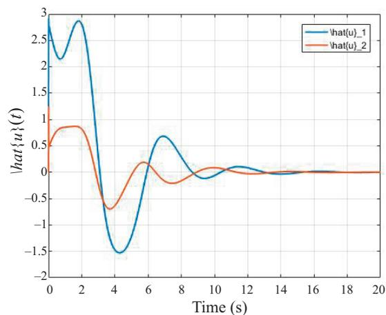
Fig. 6. Control input  $\hat{u}$  during tracking maneuver.
