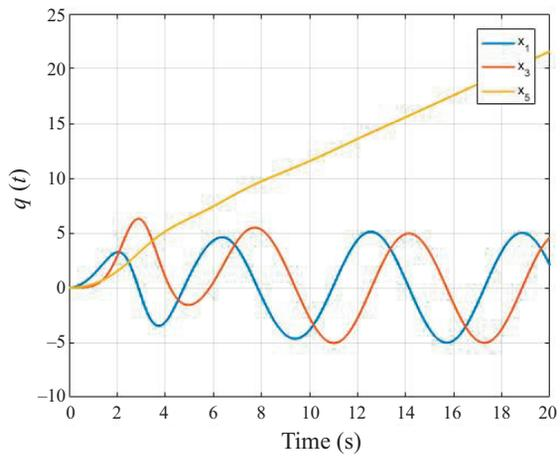
**Fig. 4.** Configuration  $q(t)$  during tracking maneuver.
