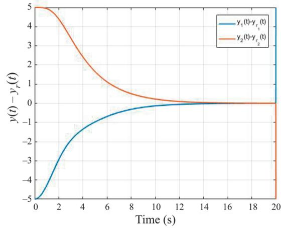
**Fig. 2.** Output error  $y(t) - y_r(t)$  during stabilization maneuver.
