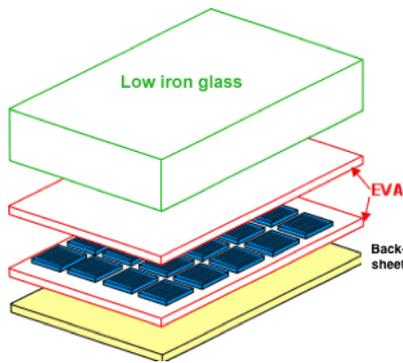
Fig. 1. Layers of solar module [8].
