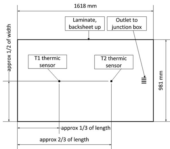
Fig. 3. Schematic representation of experimental setup.
