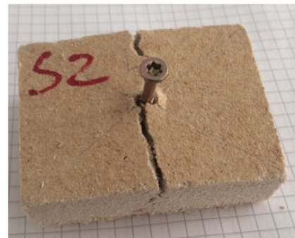
Fig. 5. Sample made by the wet method broke during the test.
