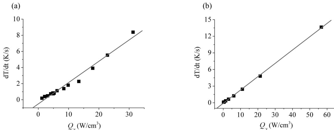
**Fig. 5.** Function  $dT/dt(Q_v)$  at start time of the AC field. Curve (a) for different frequencies ( $E_a = 840 \text{ V/mm}$ ); (b) – for different amplitudes AC ( $f = 300 \text{ Hz}$ ).
