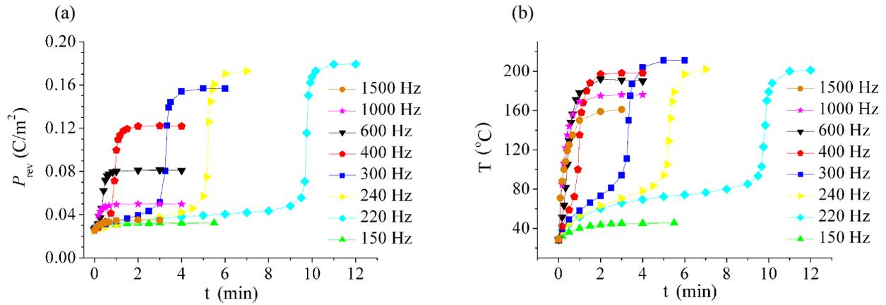
**Fig. 2.** Dependence of switched polarization (a) and heating temperature of PZT sample (b) on time during exposure electric fields of different frequencies.  $E_a = 850$  V/mm.
