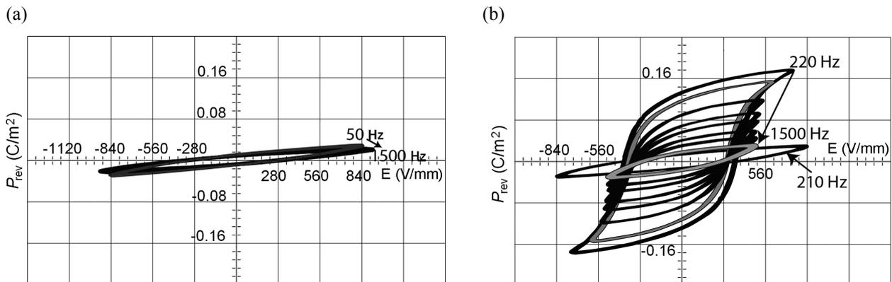
**Fig. 1.** Dielectric hysteresis loop evolution of PZT sample. (a) at the start time of field application of different frequencies; (b) maximal value.  $E_a = 850$  V/mm. Vertical ( $280 \text{ V mm}^{-1}/\text{div}$ ) and horizontal ( $0.08 \text{ C}\cdot\text{m}^{-2}/\text{div}$ ) scaling are the same for both (a) and (b) graphs.
