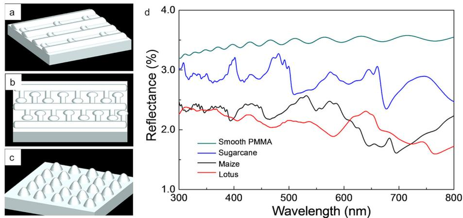
**Fig. 2.** Numerical simulation of light interference with the leaf models: (a) sugarcane model; (b) maize model; (c) lotus model; (d) simulation results of optical reflectance in the range of visible light.
