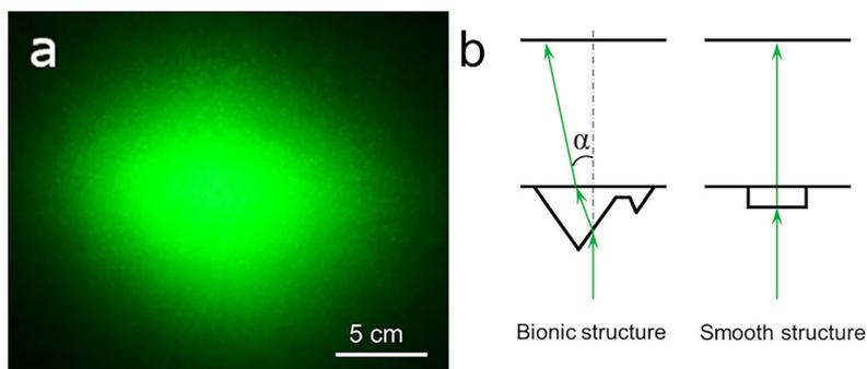
**Fig. 3.** Measurements of optical transmission haze. (a) Incident laser beam scattered by bionic maize leaf; (b) schematic diagram of light scattering.
