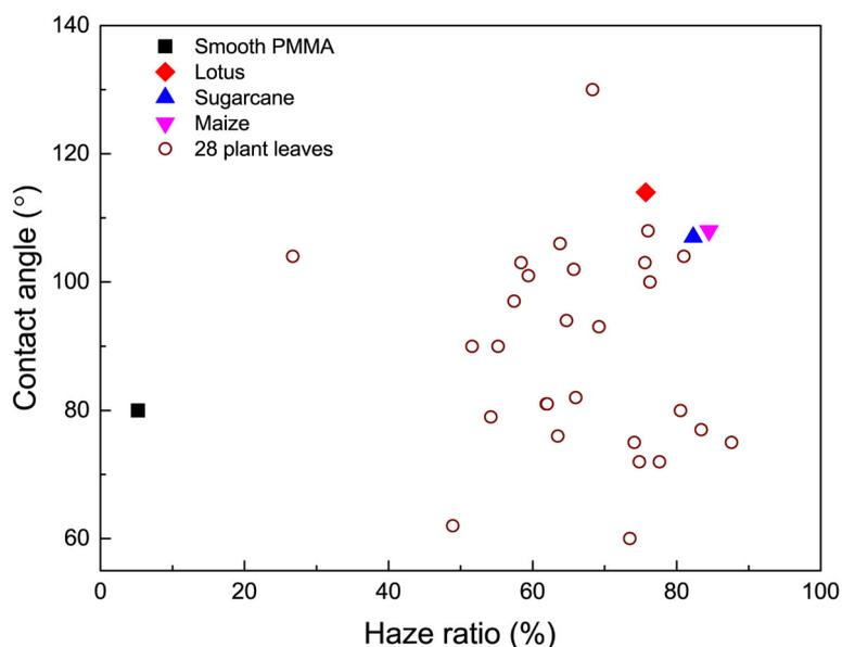
**Fig. 6.** Relationships between contact angle and haze ratio for PMMA sheets with different leaf surfaces.
