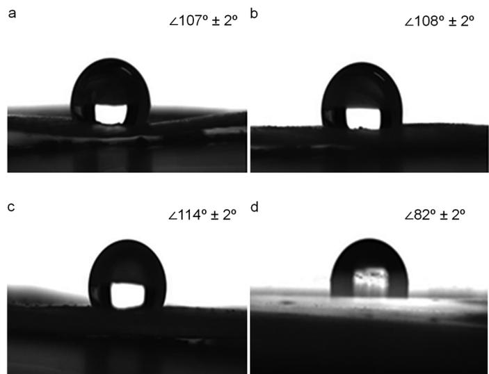
Fig. 5. Contact angle measurements of four PMMA sheets with different surfaces. Bionic structures replicated from sugarcane (a), maize (b) and lotus (c) leaves. Smooth PMMA was also measured as reference (d).
