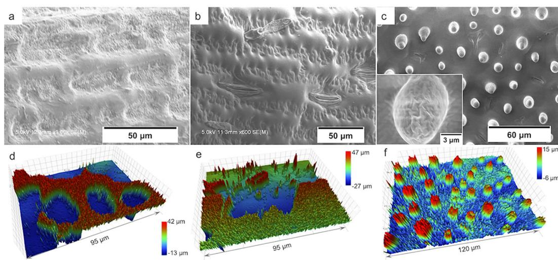
**Fig. 1.** SEM images and surface profile of replicated sugarcane, maize and lotus leaf structures. (a), (d) sugarcane; (b), (e) maize; (c), (f) lotus. The inset shows a zoomed-in image on lotus leaf. The surface profiles of randomly selected square regions (panel d, e, f) were taken on the replicated leaves but at different positions from SEM images, and the side lengths were marked in each panel.
