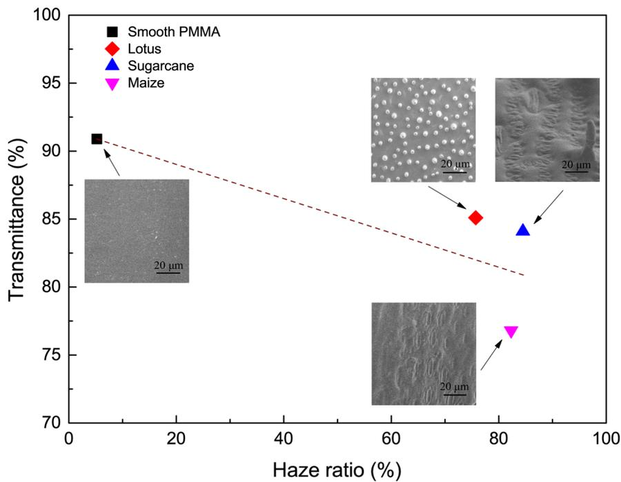
Fig. 4. Relationships between optical transmittance and haze ratio for PMMA sheets with different surface structures.
