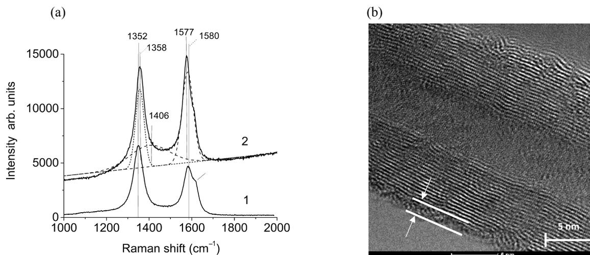
**Fig. 2.** Base-line corrected Raman spectra (a) of pristine MWCNTs (1) and P3OT-f-MWCNTs (2); and representative TEM image (b) of P3OT-f-MWCNTs.
