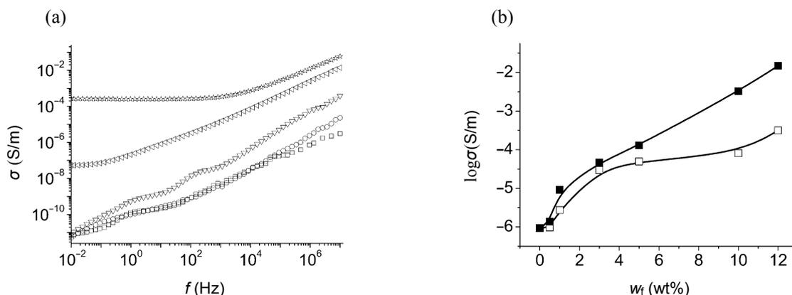
**Fig. 6.** Electrical conductivity  $\sigma$  of the selected EOC17 composites with various wt% contents of P3OT-f-MWCNTs ( $\square$  – 0%,  $\circ$  – 0.5%,  $\nabla$  – 3%,  $\triangleleft$  – 10%,  $\star$  – 12%) as a function of frequency (a); and electrical conductivity of the investigated nanocomposites with pristine (open symbols) and functionalized (closed symbols) MWCNTs at 1MHz frequency as function of the nanofiller content (b).
