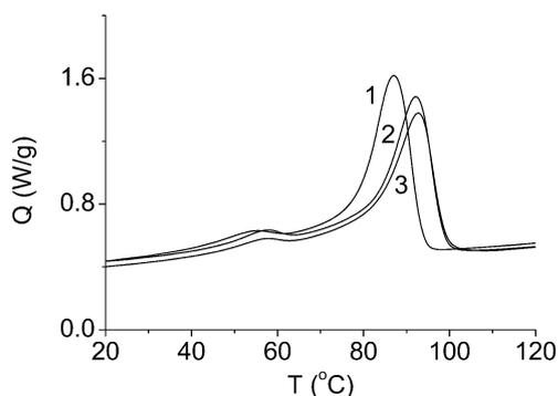
**Fig. 3.** DSC cooling traces of neat EOC17 (1) and EOC17 nanocomposites with 3 wt% of P3OT-f-MWCNTs (2) and 10 wt% of P3OT-f-MWCNTs (3).
