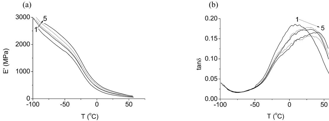
**Fig. 4.** Storage modulus  $E'$  (a) and loss tangent  $\tan\delta$  (b) of EOC17 (1) and its nanocomposites with 3 wt% of MWCNTs (2), 3 wt% of P3OT-f-MWCNTs (3), 10 wt% of MWCNTs (4) and 10 wt% of P3OT-f-MWCNTs (5).
