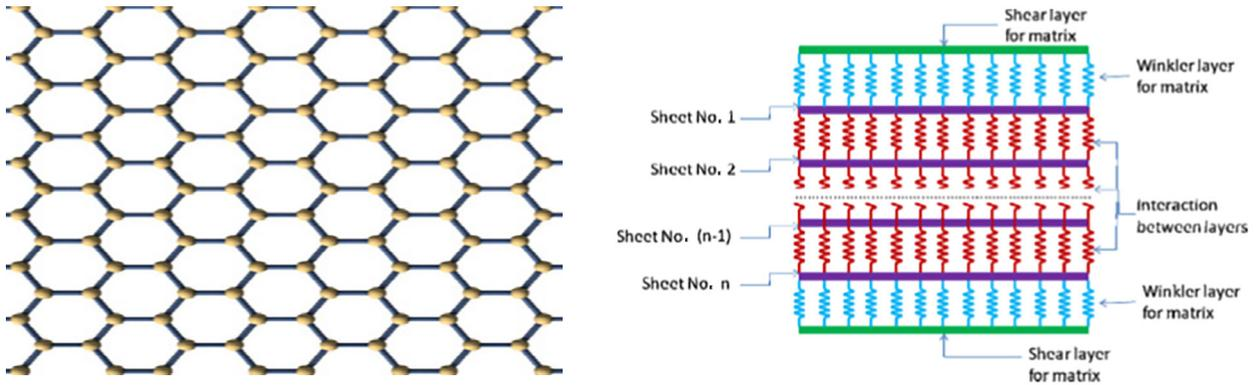
Fig. 1. (a) A single-layer graphene sheet; (b) continuum model of multilayered graphene laminate embedded in a polymer matrix [19].
