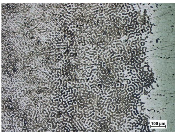
**Fig. 6.** The pattern successfully replicated on polished aluminium. The quality of this stamp is evaluated as acceptable.
