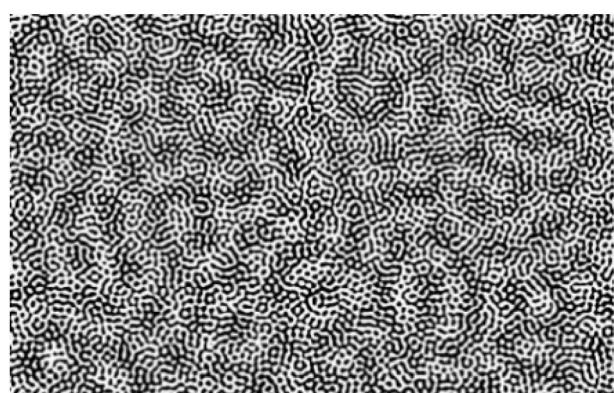
**Fig. 1.** A sample optical pattern. Actual feature dimension: 1–10 µm. The base of small features creates wave-like patterns at higher length scales [2].
