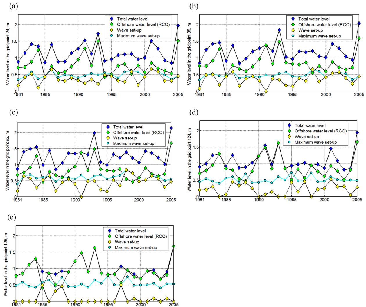
**Fig. 5.** The proportion of the wave set-up and offshore water level in the formation of annual maxima of the total water level at the shoreline at four representative sections of the study area: (a) Tiskre (section 24), (b) Pirita (85), (c) Viimsi (92), (d) Muuga (124), (e) a location close to Muuga Harbour (126) where wave set-up almost does not contribute. See Fig. 2 for the numbering of coastal sections.
