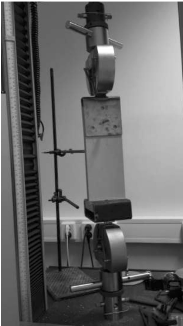
Fig. 2. Tensile test setup.
