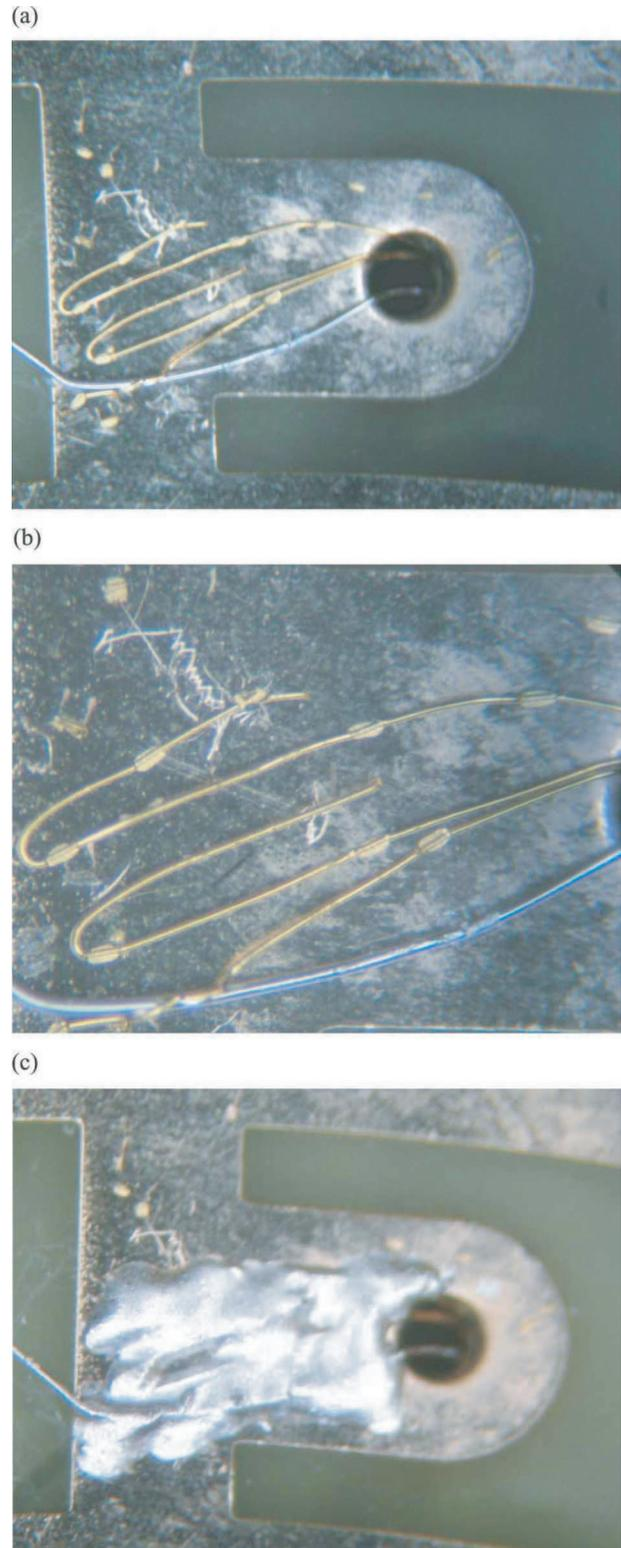
**Fig. 8.** Slip ring bond. (a) Basewire and three gold wires bonded on the slip ring. (b) Closeup of the same bonds. (c) All bonds covered with conducting glue.
