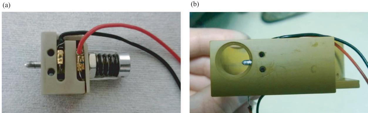
**Fig. 10.** (a) Launch lock, loaded. (b) Launch lock placed at its position in tether isolation. Notice the pin entering the end mass compartment.
