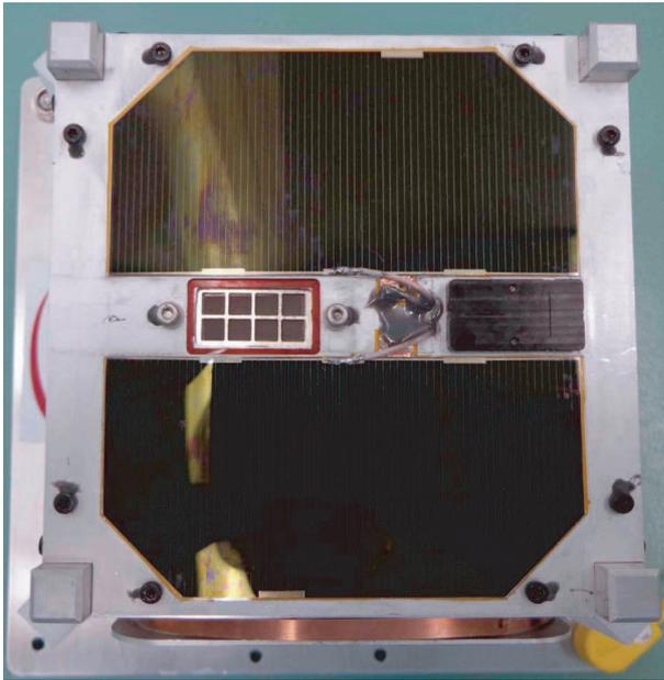
Fig. 16. Electron gun attached on the satellite side panel.
