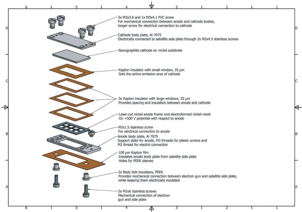
Fig. 14. Exploded view of the electron gun.
