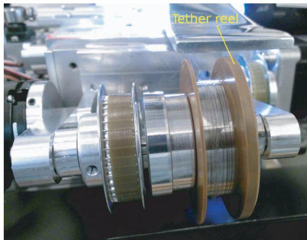
**Fig. 4.** Tether being manufactured on the reel at the UH on 15 January 2013.
