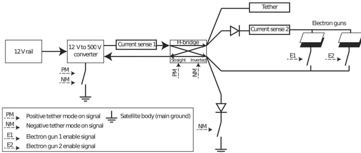
Fig. 13. Schematic presentation of the high-voltage supply.
