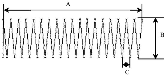
**Fig. 1.** Embroidery area formation diagram: A – length of the embroidered element = 60 mm, B – width of the embroidered element = 6.0 mm, C – stitch density = 0.42 mm.
