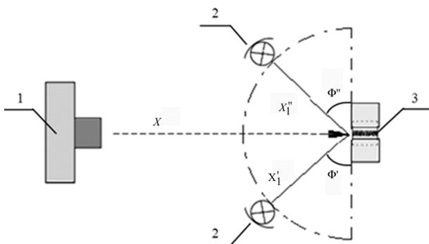
**Fig. 2.** Illustration of a photo-captured embroidered test specimen by a digital camera: 1 – digital camera; 2 – light source; 3 – test specimen. Distance between 3 and 1 is  $X \approx 0.35$  m; distance from light source 2 to test specimen 3 is  $X' = X'' \approx 0.1$  m. The angle between the test specimen and light propagation direction  $\Phi' = \Phi'' = 45^\circ$ .
