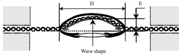
**Fig. 3.** Diagram for measuring an embroidered element: D – embroidery width, E – wave height.
