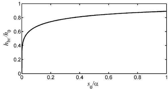
Fig. 2. Breaking depth versus wave steepness.
