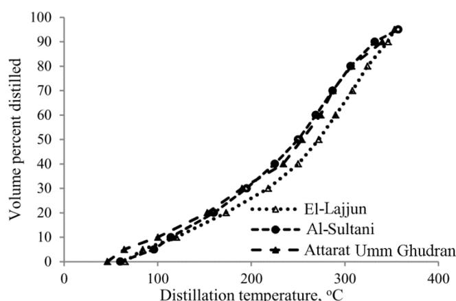
Fig. 1. Distilled shale oils volume percent as a function of distillation temperature.
