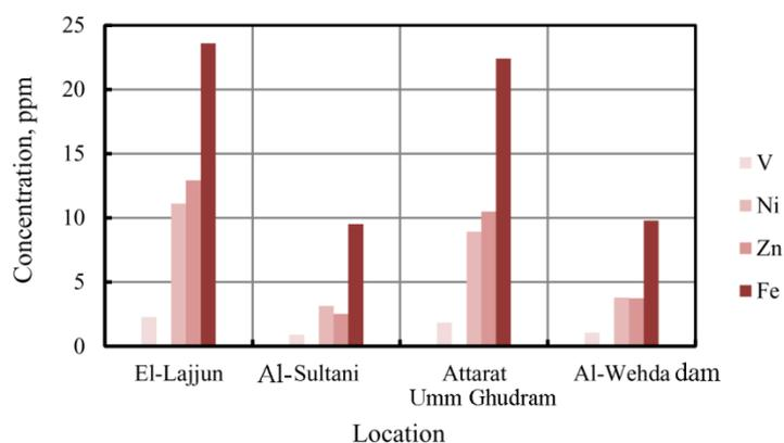
Fig. 2. Concentrations of V, Ni, Zn and Fe in shale oils by location.
