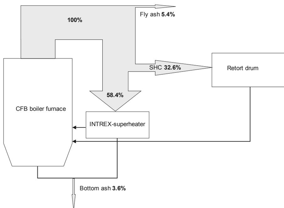
Fig. 9. The approximate relative distribution of ash flow leaving the furnace of the CFB boiler with an electrical capacity of 107.5 MW, integrated with the retort drum with an oil shale input capacity of 280 t/h. The heating value of oil shale as received is 8.4 MJ/kg and the initial temperature of SHC is 750 °C. The temperature in the INTREX superheater is in the range of 760–620 °C.
