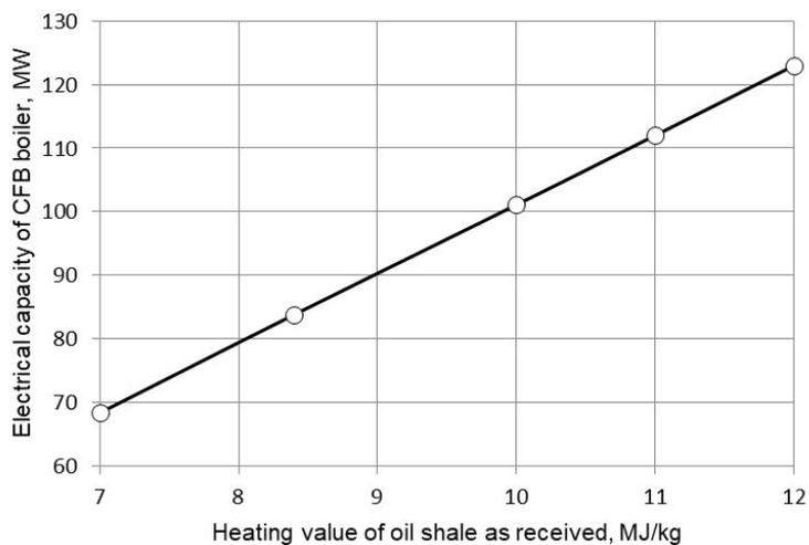
Fig. 5. The electrical capacity of the CFB boiler dependent on the heating value of oil shale as received for the integrated retort drum load of 280 t/h.
