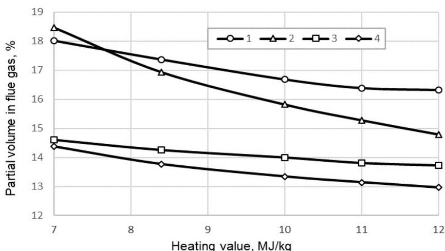
Fig. 7. The content of CO<sub>2</sub> and water vapour in the flue gas dependent on the heating value of oil shale as received. 1 – water vapour at combustion of semi-coke and retort gas; 2 – CO<sub>2</sub> at combustion of semi-coke and retort gas; 3 – water vapour at oil shale combustion; 4 – CO<sub>2</sub> at combustion of oil shale.
