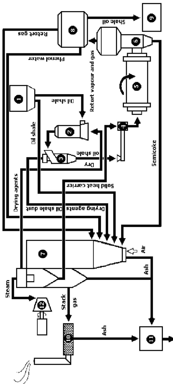
Fig. 1. SPC technology schema. 1 – oil shale storage, 2 – dryer, 3 – cyclone of dry oil shale, 4 – mixer of SHC and oil shale, 5 – rotating retort reactor, 6 – separator of oil vapour and semi-coke, 7 – CFB boiler, 8 – condenser of oil vapour, 9 – shale oil storage, 10 – flue gas cleaner, 11 – bottom and fly ash bunker, 12 – turbo-generator for power production.
