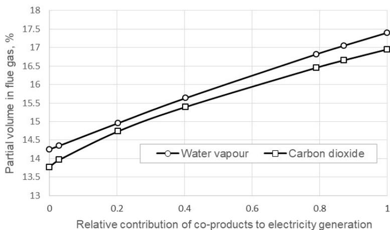
Fig. 6. The content of CO<sub>2</sub> and water vapour in the flue gas dependent on the contribution of semi-coke and retort gas to electricity generation. The heating value of oil shale as received is 8.4 MJ/kg.
