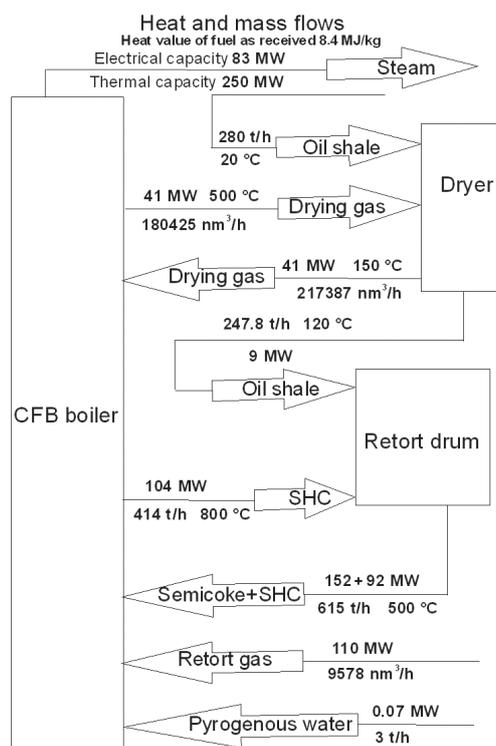
Fig. 3. The heat and mass fluxes in the SPC unit consisting of the CFB boiler and the retort drum with an oil shale input capacity of 280 t/h firing only co-products of oil shale retorting. The extent of carbonate decomposition is 0.7. The heat loss with bottom ash is 9.3 MW and the quantity of heat leaving the condenser with cooling water is 18.3 MW. The quantity of heat entering the furnace of the CFB boiler with semi-coke consists of its heat of combustion (152 MW) and sensible heat.
