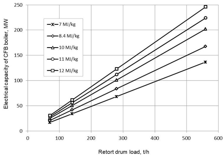
Fig. 4. The electrical capacity of the CFB boiler dependent on the load of the integrated retort drum and the heating value of oil shale as received, if exclusively the co-products of the oil shale retorting process were fired.
