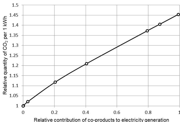
Fig. 8. The relationship between the quantity of CO<sub>2</sub> per one kWh of produced electricity in the application of SPC technology to the quantity of CO<sub>2</sub> per one kWh of produced electricity in burning only oil shale dependent on the contribution of co-products to electricity production.
