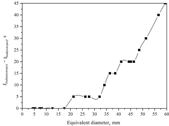
Fig. 7. Change of the final heating time difference between isotropic and anisotropic oil shale particles with equivalent diameter.
