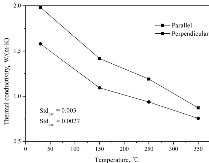
Fig. 1. Changes of thermal conductivity with temperature.
