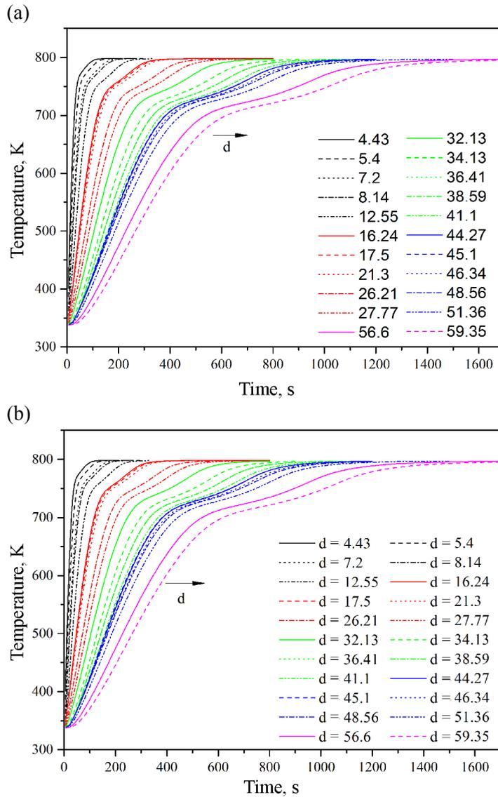
Fig. 5. Heating time of oil shale (a) with average thermal conductivity, (b) with different thermal conductivities.
