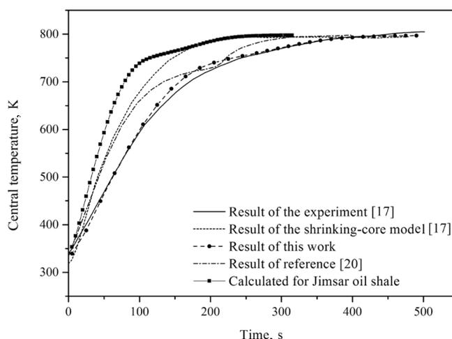
Fig. 4. Comparison of calculated and experimental central temperature history data on oil shale.
