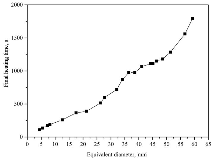
Fig. 8. Change of the final heating time of anisotropic oil shale with particle equivalent diameter.
