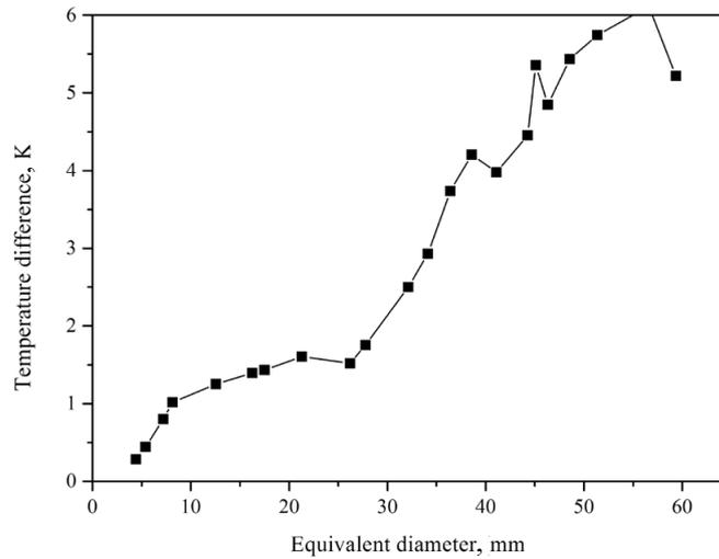
Fig. 6. Change of the maximum temperature difference between isotropic and anisotropic oil shale particles with equivalent diameter.
