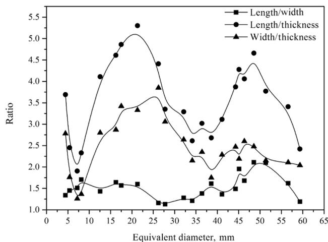
Fig. 2. Ratios of three dimensions for crushed Jimsar oil shale particles.
