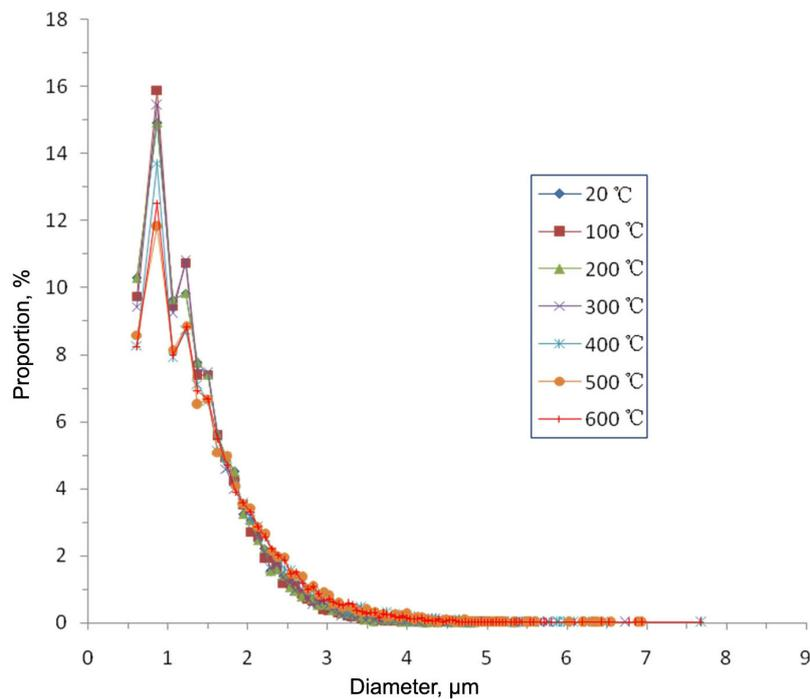
Fig. 8. Variations in the proportion of  $\mu\text{m}$ -sized pores in the oil shale sample with pore diameter at different temperatures.
