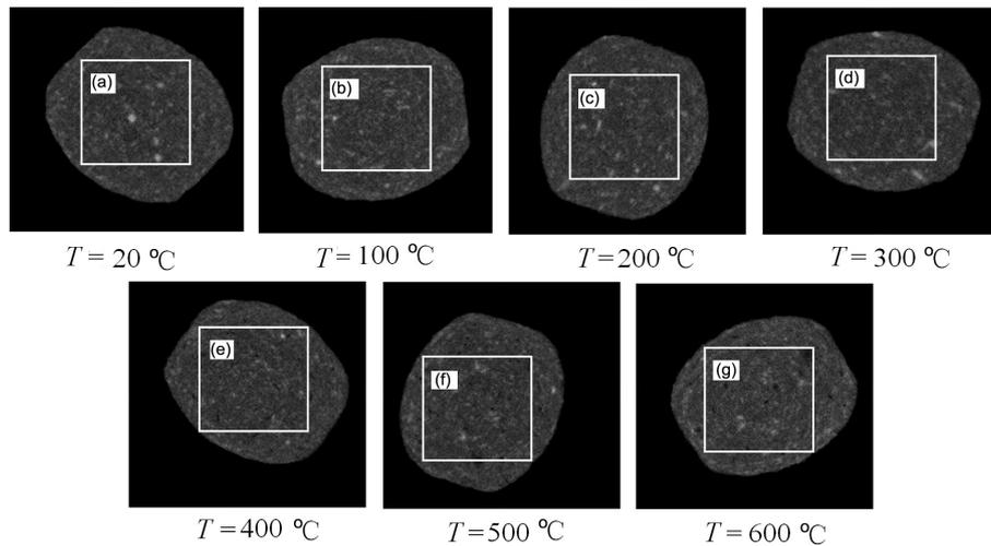
Fig. 4. CT scan grayscale images of the oil shale sample at different temperatures.
