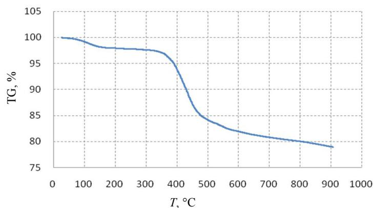
Fig. 2. TG curve of the Fushun oil shale sample at a heating rate of 15 °C/min.
