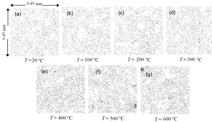
Fig. 5. The  $\mu\text{m}$ -sized pore structure of the oil shale sample obtained after binarization at different temperatures.
