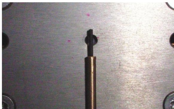
Fig. 3. The cylinder-shaped sample of oil shale ( $\varphi = 0.82 \times 7$  mm).
