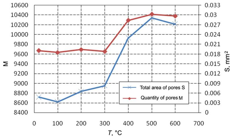
**Fig. 6.** Variations in the quantity and total area of pores in the oil shale sample with temperature.
