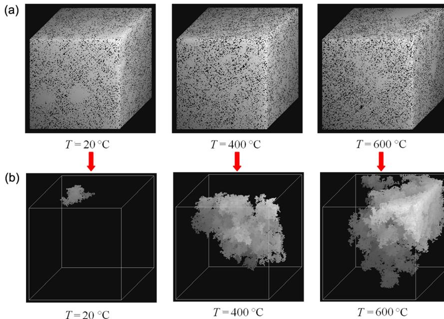
Fig. 9. (a) 3D grayscale images of the oil shale sample ( $0.22 \times 0.22 \times 0.22 \text{ mm}^3$ ); (b) the largest pore cluster at different temperatures.
