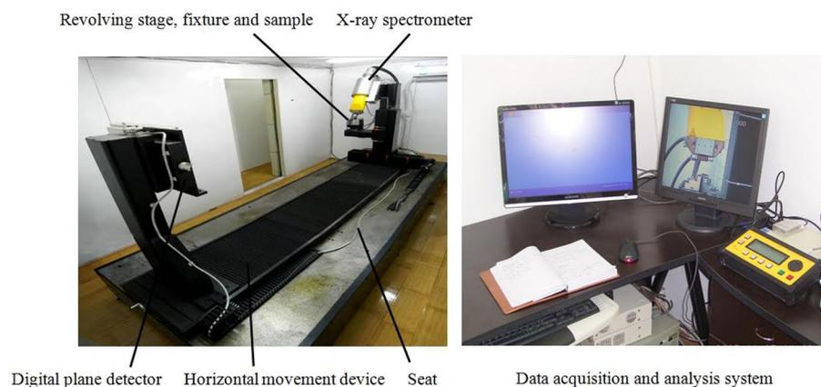
Fig. 1. Experimental micro-CT system.
