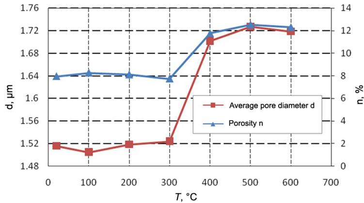
Fig. 7. Variations in the average pore diameter and porosity of the oil shale sample with temperature.
